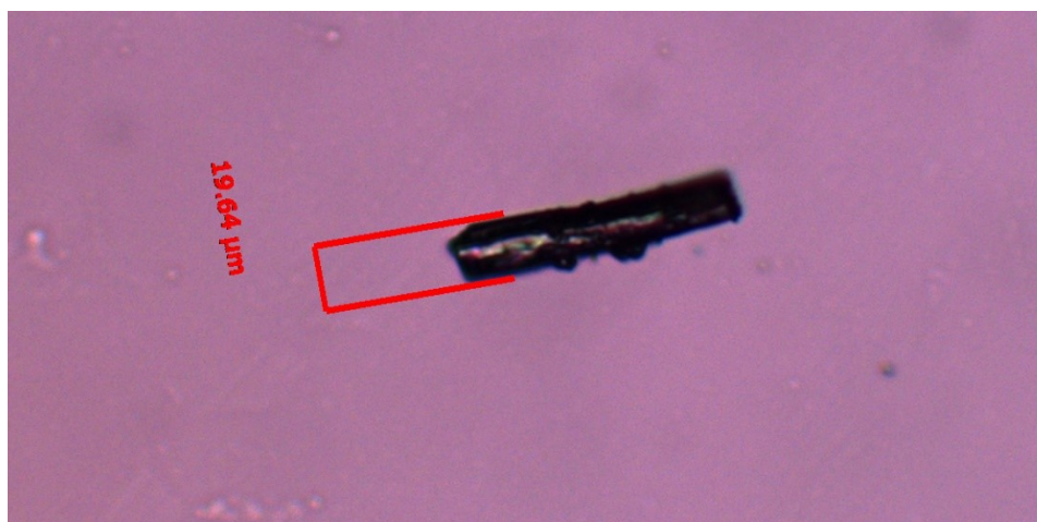
Figure S7. Single crystal of NPNH under the polarizing microscope. The measured thickness of NNPH is 19.64 \mu\text{m} .
