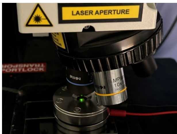
Fig. S36. Digital photographs of an in-situ Raman equipment.
