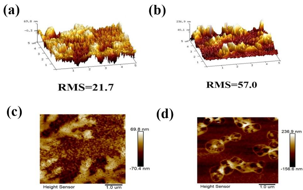
**Figure S5:** AFM topography of (a, c)  $\text{NH}_4\text{Cl}$ -20, and b, d)  $\text{NH}_4\text{Cl}$ -50 doped PEDOT: PSS
