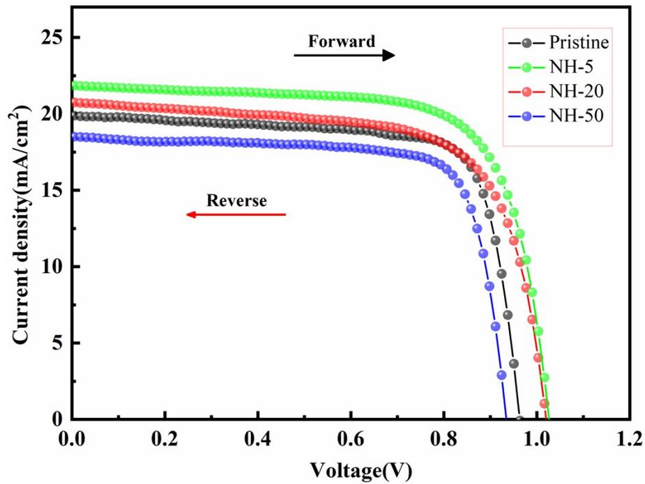
**Figure S1.** Typical J-V curves of the PSCs based on pristine and various concentrations of  $\text{NH}_4\text{Cl}$ -doped PEDOT:PSS.
