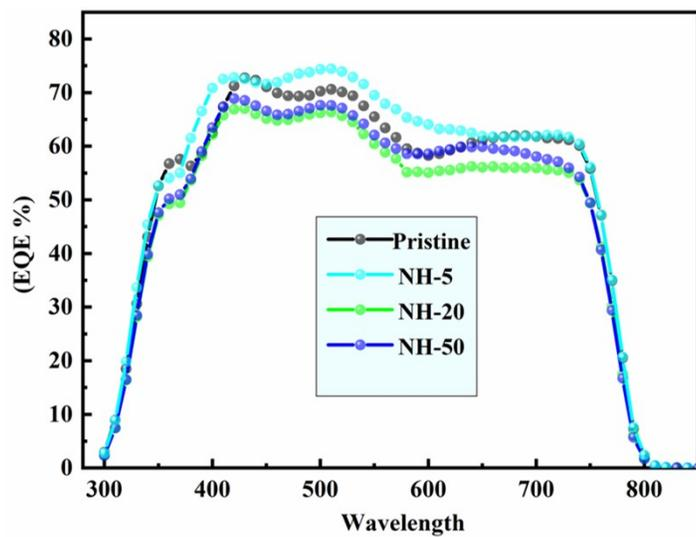
**Figure S2.** EQE spectra of the pristine and various concentration of  $\text{NH}_4\text{Cl}$ -doped PEDOT: PSS.
