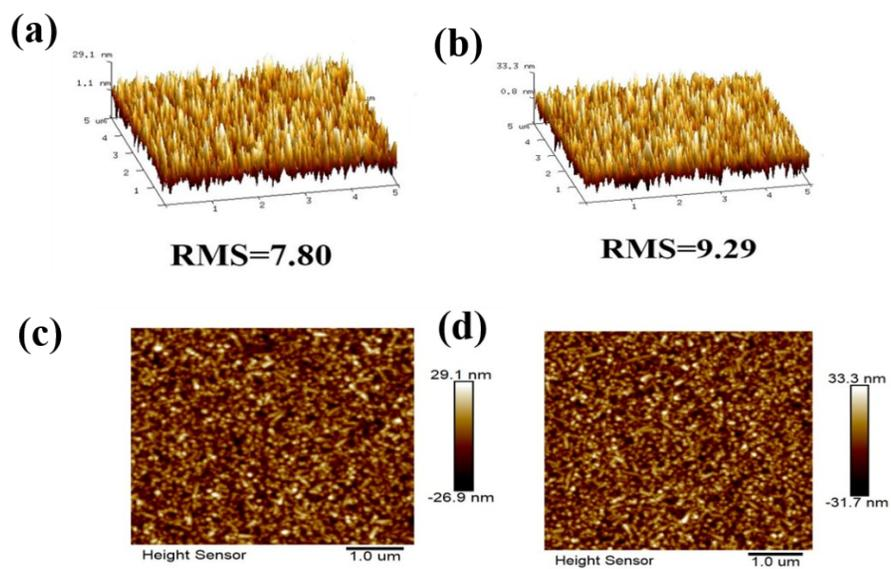
**Figure S4:** AFM topography of (a, c) Pristine, and b, d)  $\text{NH}_4\text{Cl}$ -5 doped PEDOT
