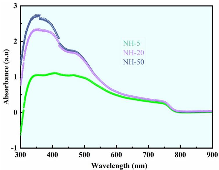
**Figure S3.** UV-visible absorbance spectra of the pristine and various concentration of NH<sub>4</sub>Cl-doped PEDOT: PSS.
