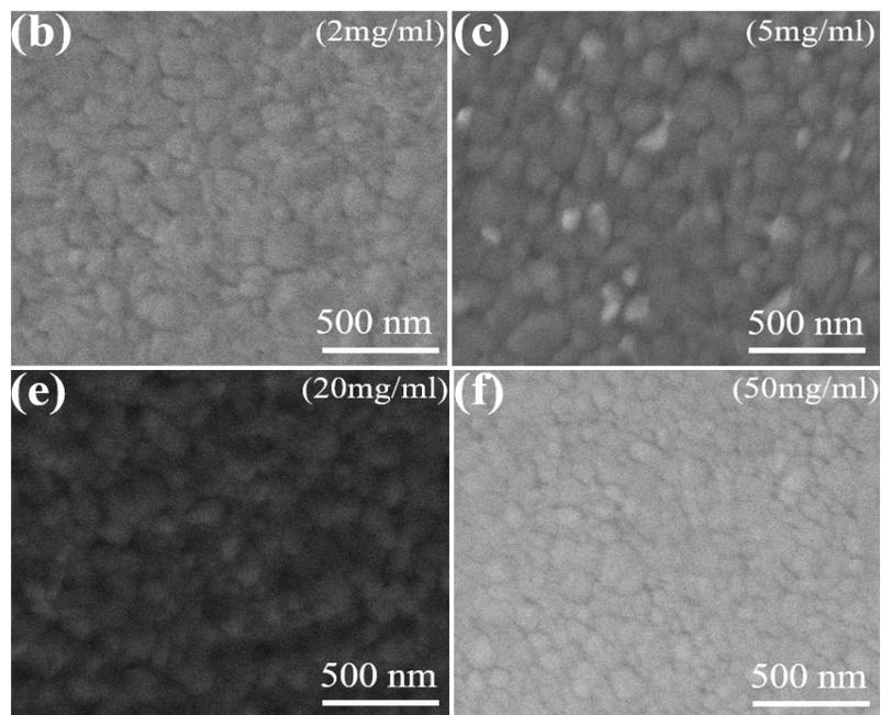
**Figure S6:** SEM images of perovskite films deposited on, (a)  $\text{NH}_4\text{Cl}$ -2, b)  $\text{NH}_4\text{Cl}$ -5, c)  $\text{NH}_4\text{Cl}$ -20, and d)  $\text{NH}_4\text{Cl}$ -50 PEDOT: PSS
