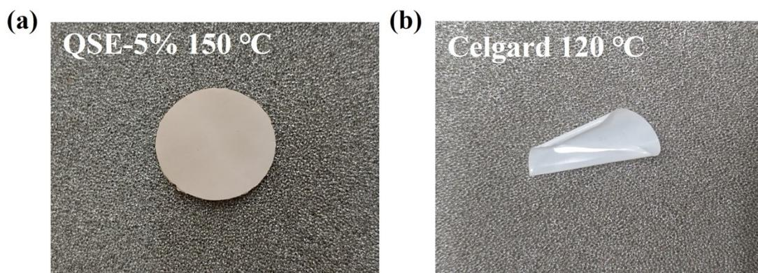
Fig. S7 Thermal stability test: (a) QSE-5%; (b) commercial electrolyte membrane (Celgard).
