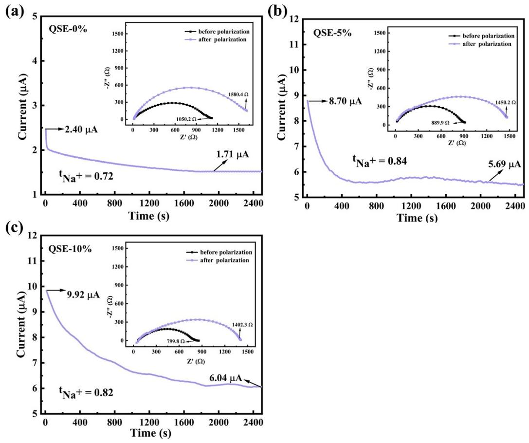
Fig. S10 The  $t_{Na^+}$  test of different QSE: (a) QSE-0%; (b) QSE-5%; (c) QSE-10%.
