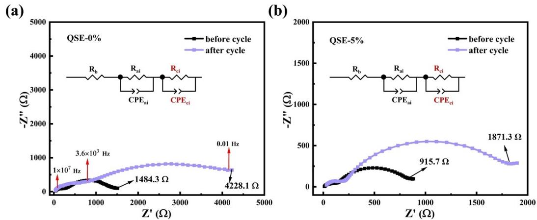
Fig. S11 Impedance test curves of quasi-solid-state sodium-ion batteries before and after cycling:
