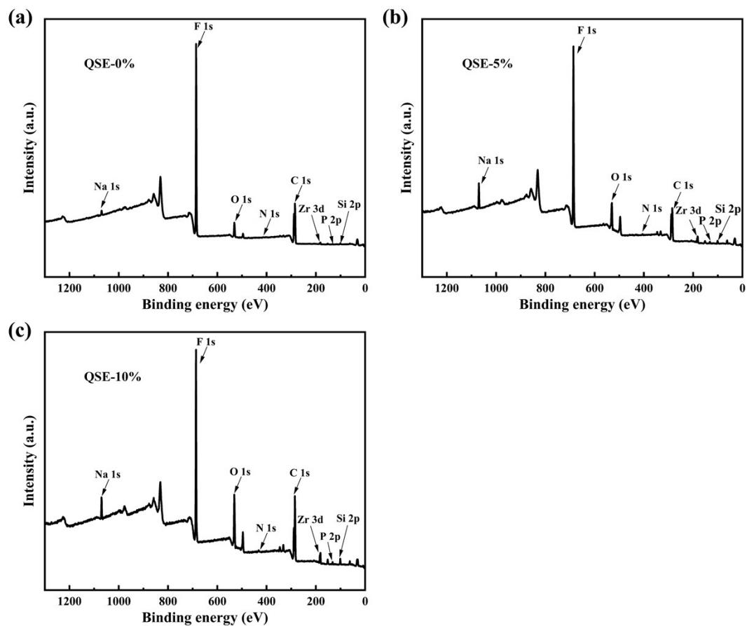
Fig. S6 XPS spectrum: (a) QSE-0%; (b) QSE-5%; (c) QSE-10%.
