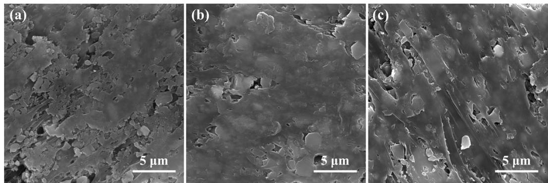
Fig. S3 The SEM images of the cross-section of (a) ASE-0%, (b) ASE-5%, and (c) ASE-10%.
