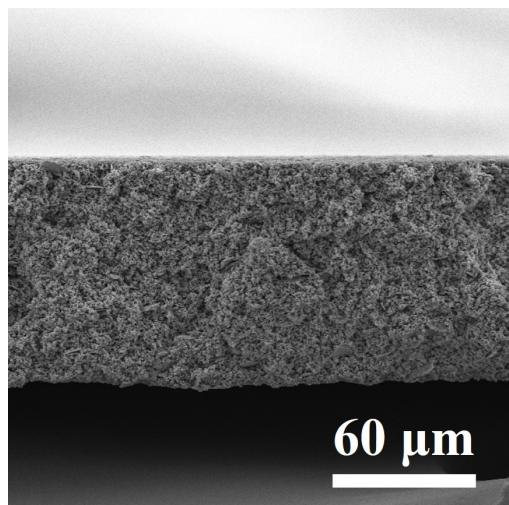
Fig. S2 SEM images of ASE-0% cross-section.
