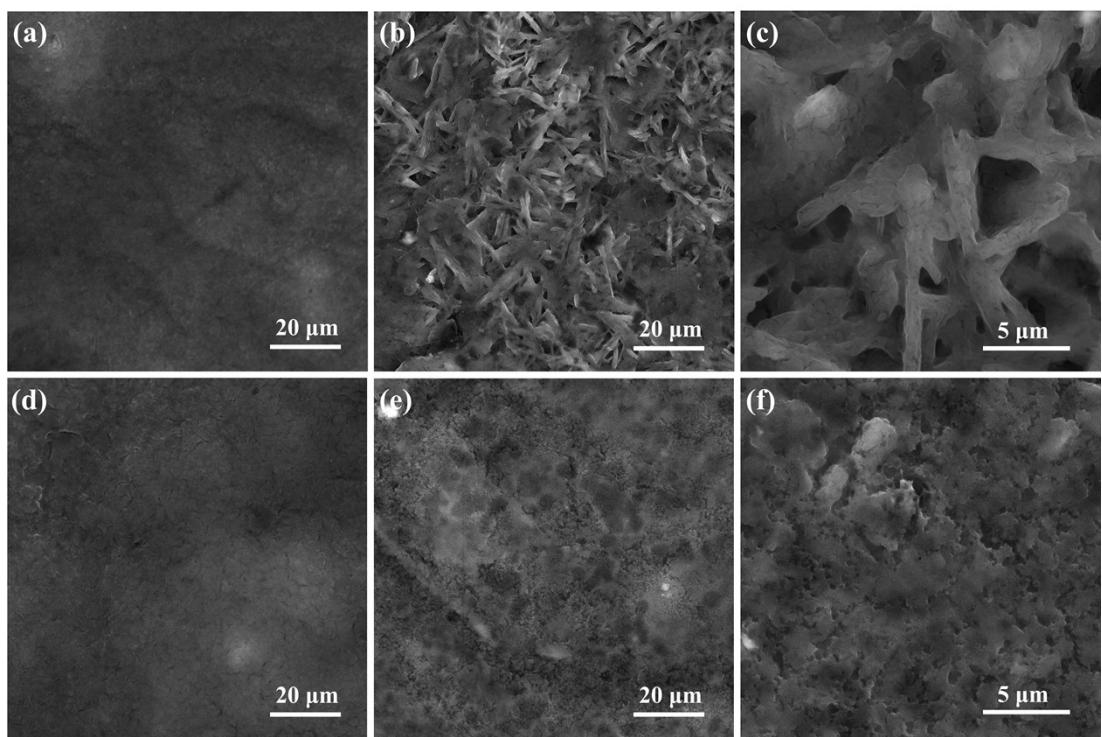
Fig. S9 SEM of sodium electrode of  $\text{Na} \mid \text{QSE-0\%} \mid \text{Na}$  battery: (a) before cycle; (b) and (c) after 1080 cycles; SEM of sodium electrode of  $\text{Na} \mid \text{QSE-5\%} \mid \text{Na}$  battery: (d) before cycle; (e) and (f) after 7500 cycles.
