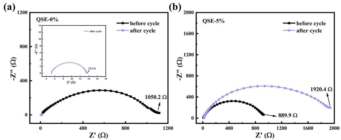
Fig. S8 Impedance test of symmetrical sodium battery before and after cycling: (a)  $\text{Na} \mid \text{QSE-0\%} \mid \text{Na}$  battery; (b)  $\text{Na} \mid \text{QSE-5\%} \mid \text{Na}$  battery.
