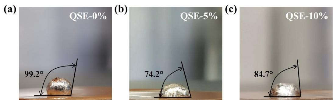
Fig. S5 Contact Angle test: (a) QSE-0%; (b) QSE-5%; (c) QSE-10%.
