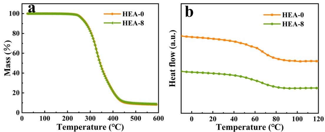
Figure S7. Thermal properties of cured HEA-0 and HEA-8 films (a. TGA curves, b. DSC curves).
