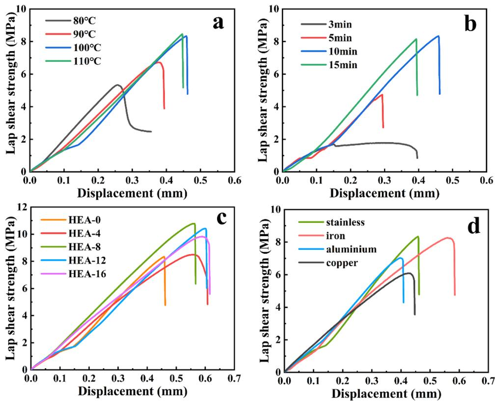
**Figure S4.** Lap shear strength-displacement curves of adhesive (a. HEA-0 on stainless steel with different bonding temperatures, b. HEA-0 on stainless steel with different bonding times, c. HEA-x on stainless steel, d. HEA-0 on different substrates).
