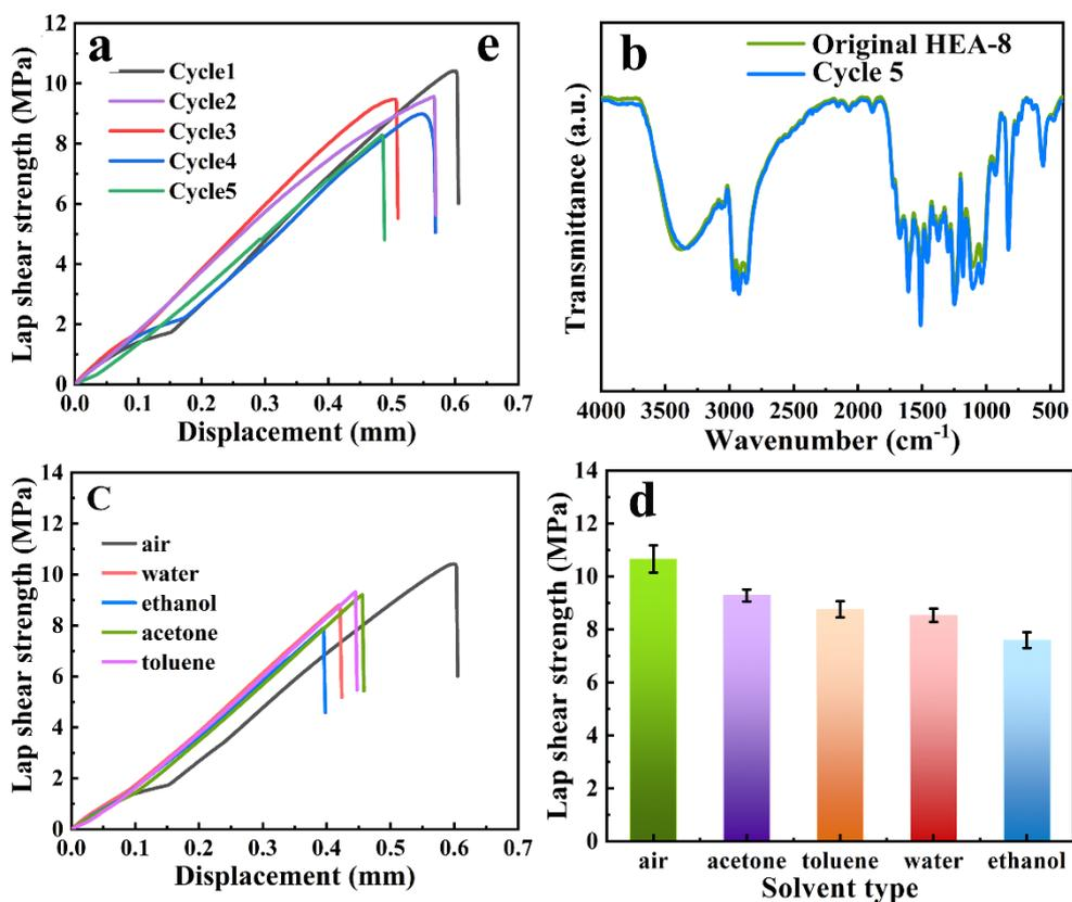
**Figure S8.** Multi-reused properties of HEA-8 (a. lap shear strength after various cycles, b. FT-IR spectra of original HEA-8 and 5<sup>th</sup> cycled HEA-8, and c-d. lap shear strength after soaking in various solvents for 72 h at room temperature).
