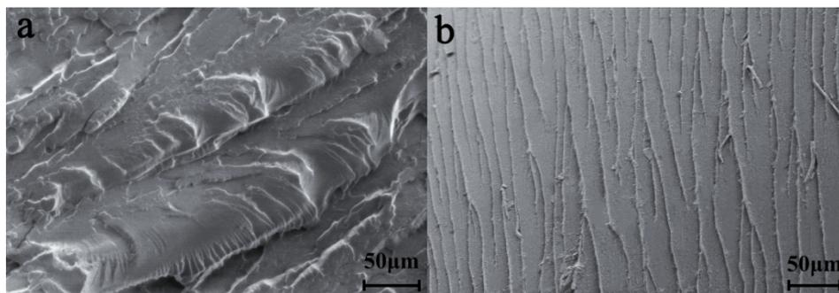
**Figure S5.** SEM images of the fracture surfaces (a. HEA-0, and b. HEA-8).
