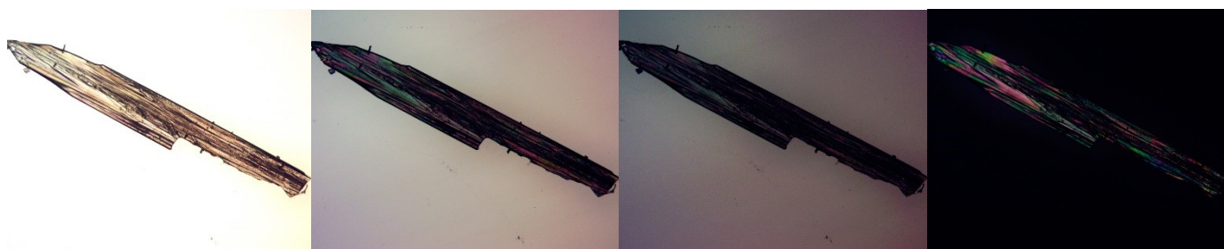
Fig. S22. Photographs of single-crystal of 1 under cross-polarized light illumination at different angle between polarizers ( 0^\circ , 30^\circ , 60^\circ , 90^\circ )
