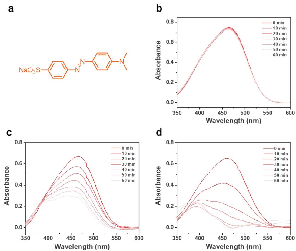
**Fig. S17** (a) The structure scheme of methyl orange. Time-dependent UV-Vis absorption spectra of MO (10 ppm) in aqueous solution upon white LED lamp irradiation ( $50 \text{ mW/cm}^2$ ) (b) without/with (c) **PNP** and (d) **Pt@PNP** (0.1 mg/mL).
