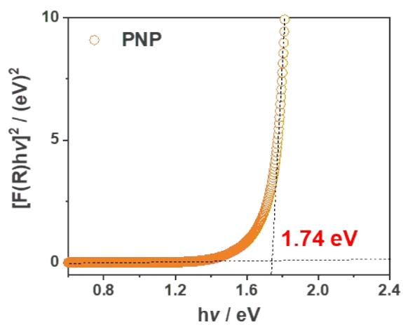
Fig. S11 The optical band gap of PNP from ssUV-vis reflectance spectra.
