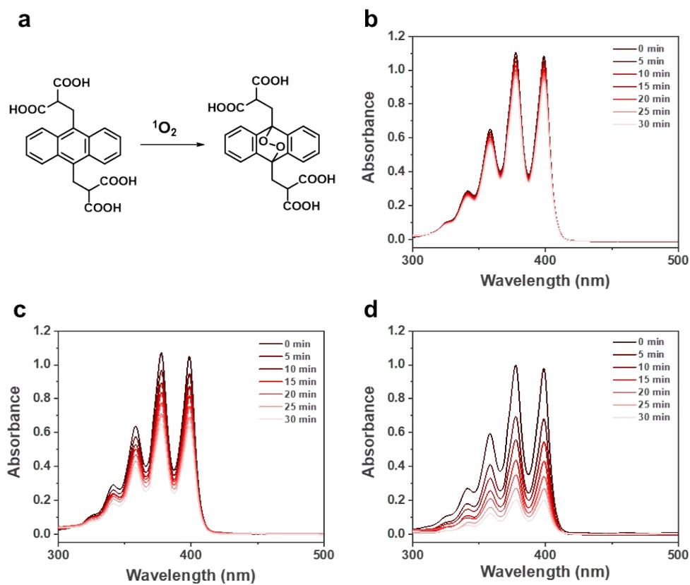
**Fig. S13** (a) The reaction scheme of ABDA with singlet oxygen. Time-dependent UV-Vis absorption spectra of ABDA (100  $\mu\text{M}$ ) in 1% DMSO/water solution upon white LED lamp irradiation (50  $\text{mW}/\text{cm}^2$ ) (b) without/with (c) PNP and (d) Pt@PNP (0.1 mg/mL).
