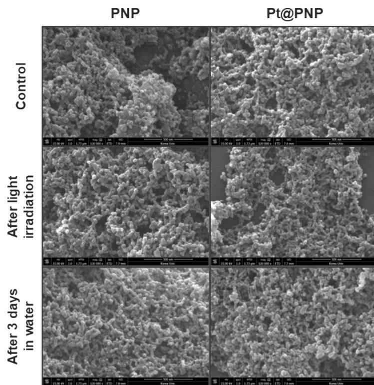
Fig. S8 SEM images of PNP and Pt@PNP for checking stability under light irradiation for 2 h and in water for 3 days.
