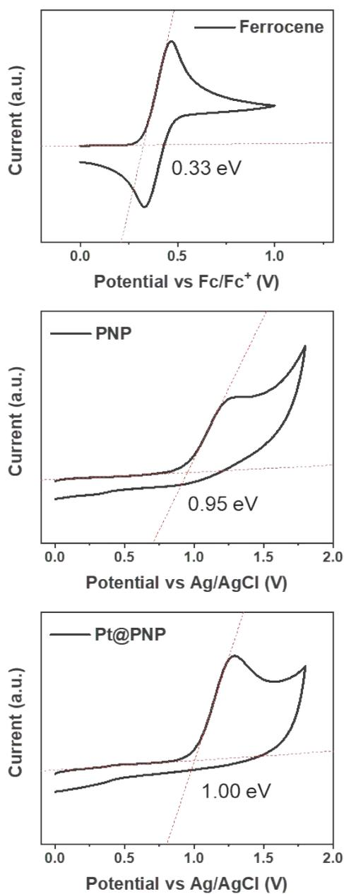
**Fig. S12** Cyclic voltammetry data of ferrocene as a reference, **PNP**, and **Pt@PNP** to measure the energy level of polymers. Before the measurement of the energy level of polymers, the experiment was conducted using ferrocene as a reference in anhydrous acetonitrile with tetrabutylammonium hexafluorophosphate (0.1 M). The working electrode was prepared by drop-casting water/isopropyl alcohol suspension of POP with 5 wt% Nafion.
