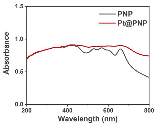
Fig. S10 Solid-state UV-vis spectra of PNP and Pt@PNP.
