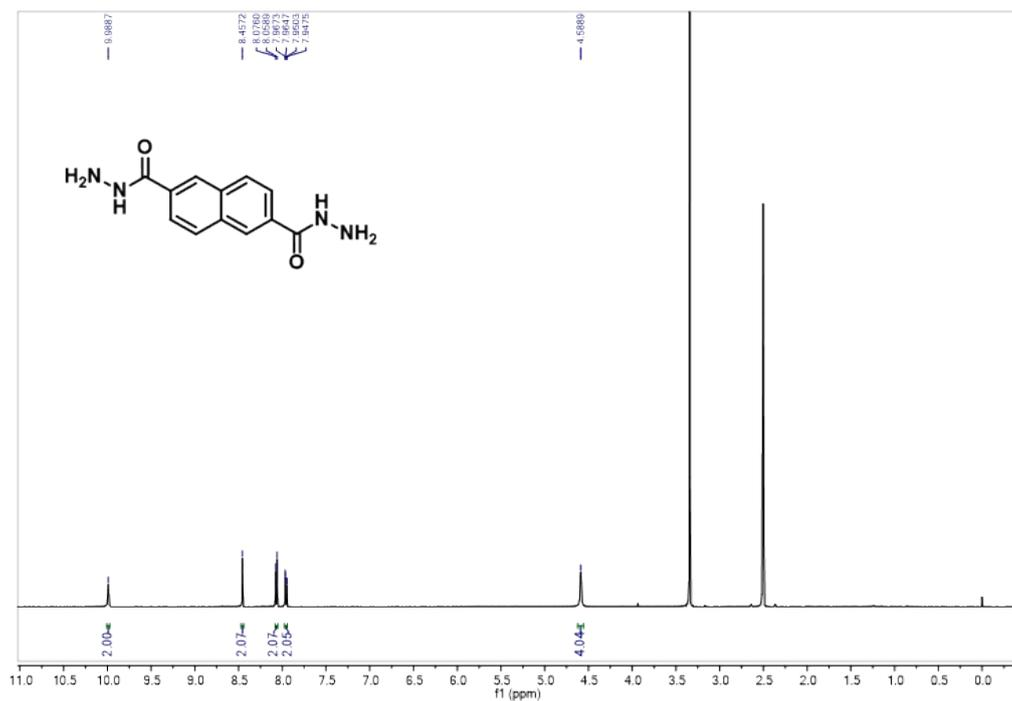
**Fig. S1** <sup>1</sup>H NMR (DMSO, 500 MHz) spectrum of NPDH
