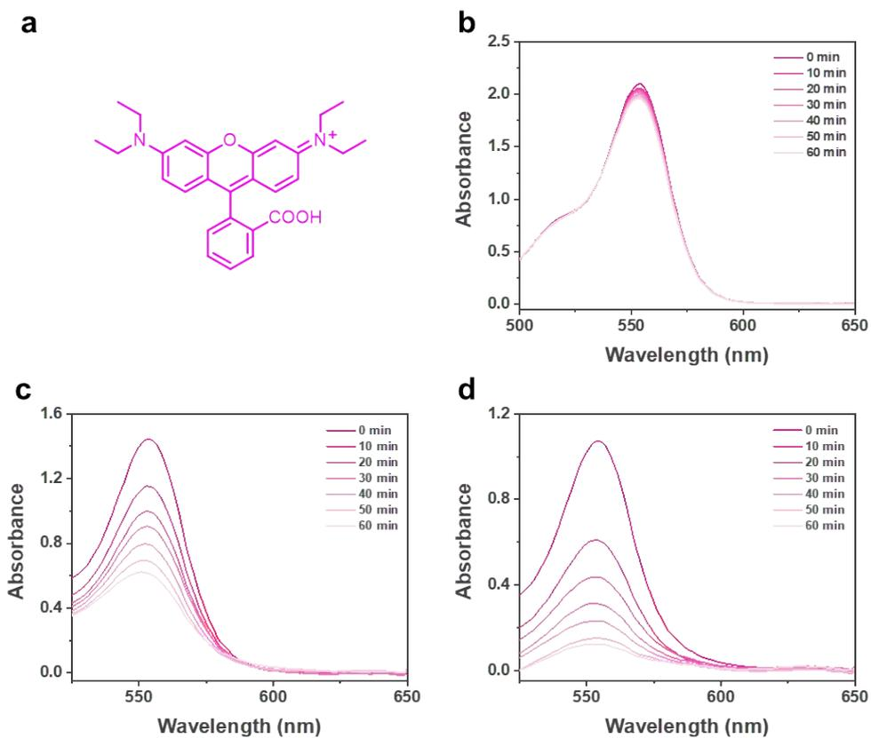
**Fig. S18** (a) The structure scheme of rhodamine B. Time-dependent UV-Vis absorption spectra of Rh B (10 ppm) in aqueous solution upon white LED lamp irradiation (50 mW/cm<sup>2</sup>) (b) without/with (c) **PNP** and (d) **Pt@PNP** (0.1 mg/mL).
