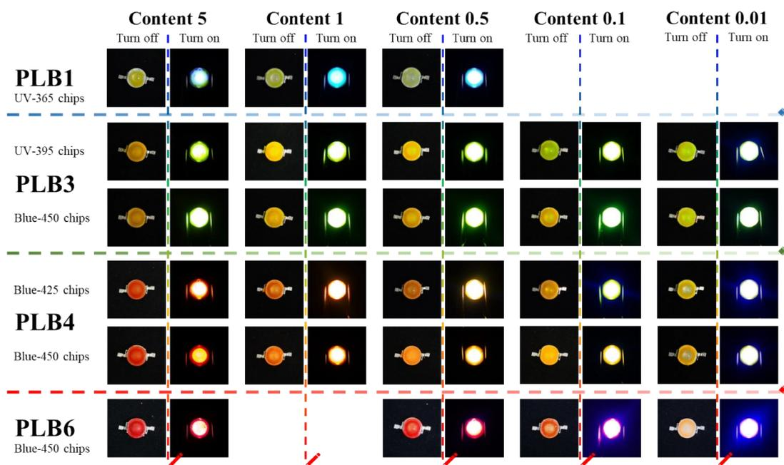
**Fig. S5.** Turn on and turn off photos of the LEDs prepared by **PLB1**、**PLB3**、**PLB4** and **PLB6** on different doping amounts and different excitation chips. The content is the doping mass (mg) of each compound in 110 mg (100 mg A glue +10 mg B glue) AB glue.
