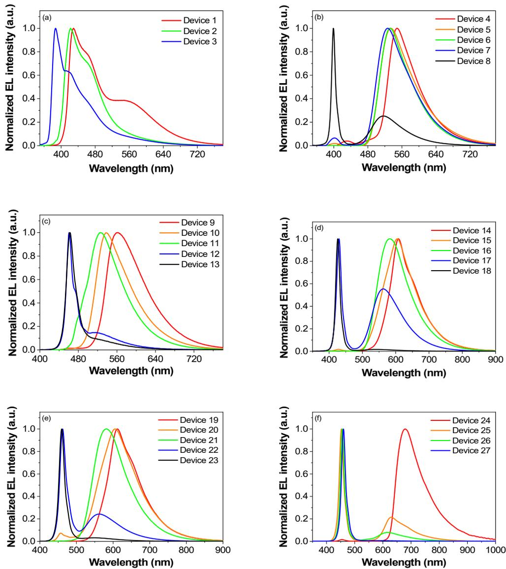
**Fig. S6.** (a) Spectra of devices made from **PLB1** and UV-365 chips. (b) Spectra of devices made from **PLB3** and UV-395 chips. (c) Spectra of devices made from **PLB3** and Blue-450 chips. (d) Spectra of devices made from **PLB4** and Blue-425 chips. (e) Spectra of devices made from **PLB4** and Blue-450 chips. (f) Spectra of devices made from **PLB6** and Blue-450 chips.
