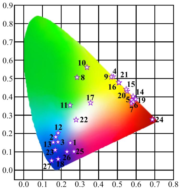
Fig. S7. The chromaticity coordinate chart of LED Devices.
