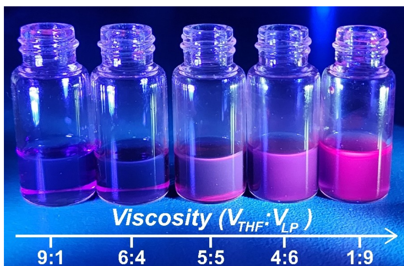
Figure S19. The emission picture of POZ-PZ in THF and liquid paraffin (LP) combination.
