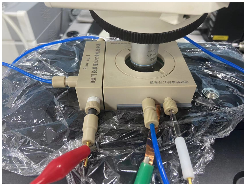
Figure S20. The optical photograph of the in-situ Raman device for urea electroanalysis.
