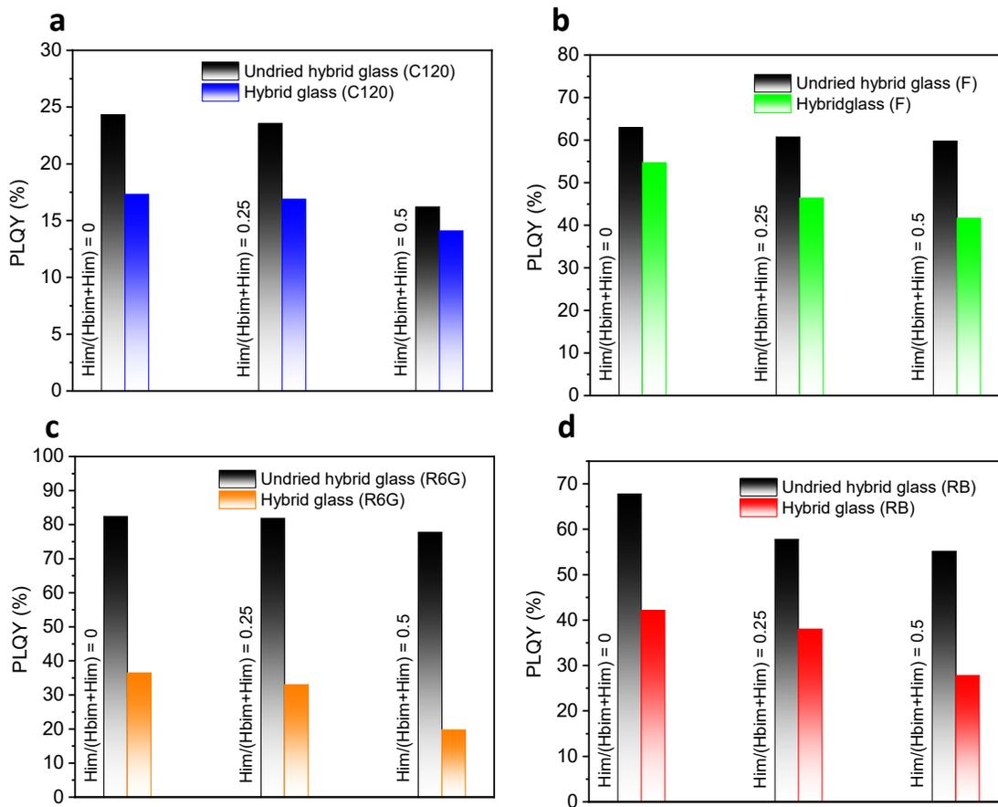
**Fig. S25.** PLQY of the undried hybrid glasses and hybrid glasses doped with **a**, C120, **b**, F, **c**, R6G, and **d**, RB at  $\text{Him}/(\text{Hbim}+\text{Him}) = 0, 0.25, \text{ and } 0.5$ .
