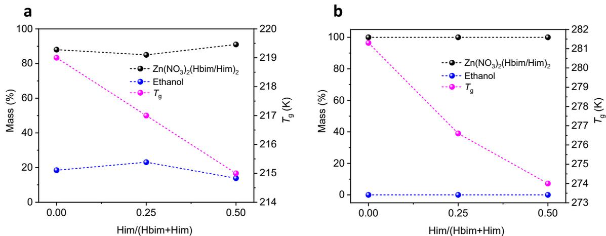
**Fig. S15.** The composition of the as-synthesized glasses and the  $T_g$  value as a function of the organic linkers ratio for **a**, undried hybrid glasses and **b**, brown hybrid glasses.
