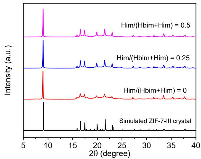
**Fig. S3.** PXRD patterns of the ZIF-7-III crystal at  $\text{Him}/(\text{Hbim}+\text{Him}) = 0, 0.25,$  and  $0.5$  synthesized by the solvothermal method.
