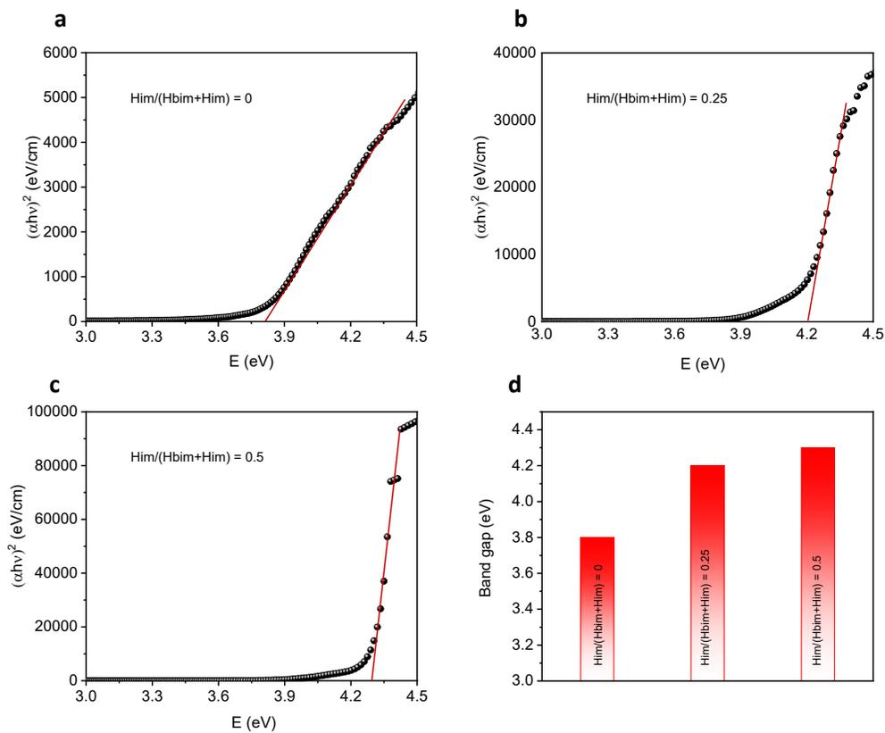
**Fig. S18.** Tauc's plot of the hybrid glasses at **a**,  $H_{im}/(H_{bim}+H_{im}) = 0$ , **b**,  $H_{im}/(H_{bim}+H_{im}) = 0.25$ , and **c**,  $H_{im}/(H_{bim}+H_{im}) = 0.5$ . **d**, Dependence of the band gap of glass on the organic linkers ratio.
