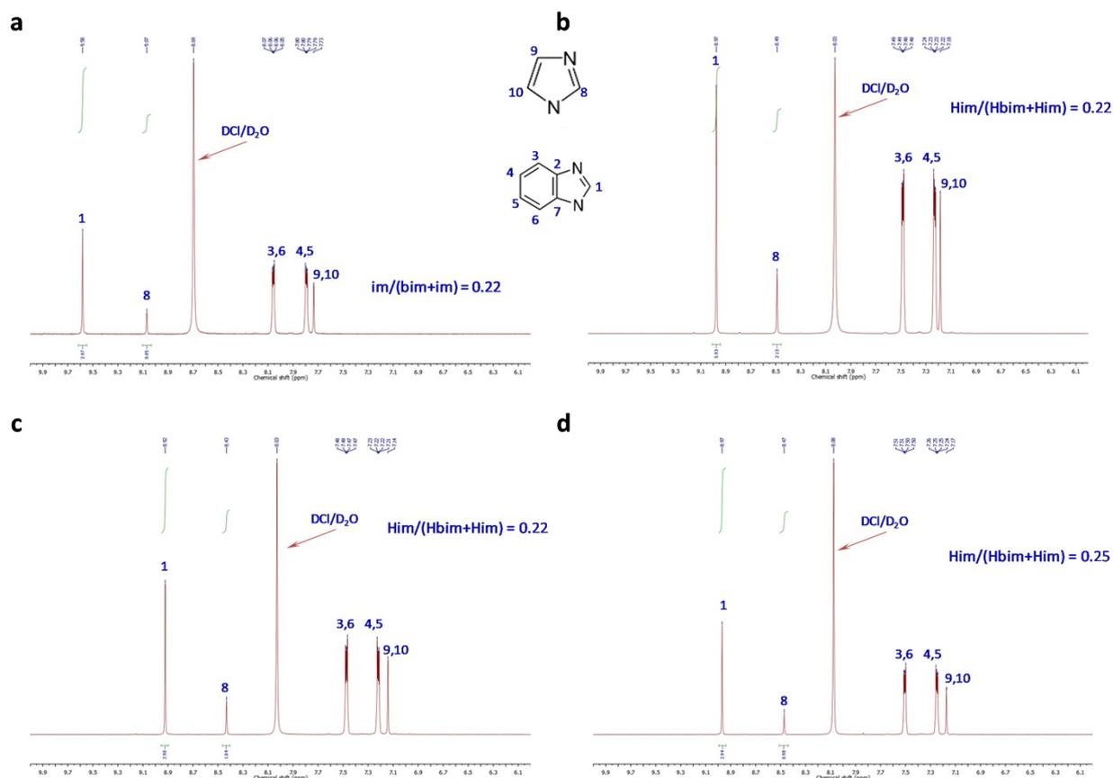
**Fig. S11.** Solution  $^1\text{H-NMR}$  spectra of the **a**, ZIF-7-III crystal, **b**, undried hybrid glass, **c**, hybrid glass, and **d**, brown hybrid glass at  $\text{Him}/(\text{Hbim}+\text{Him}) = 0.25$ . The normalized proton integration values and the proton peak positions are in green and blue colors, respectively. The insets are the molecular structures of Him and Hbim.
