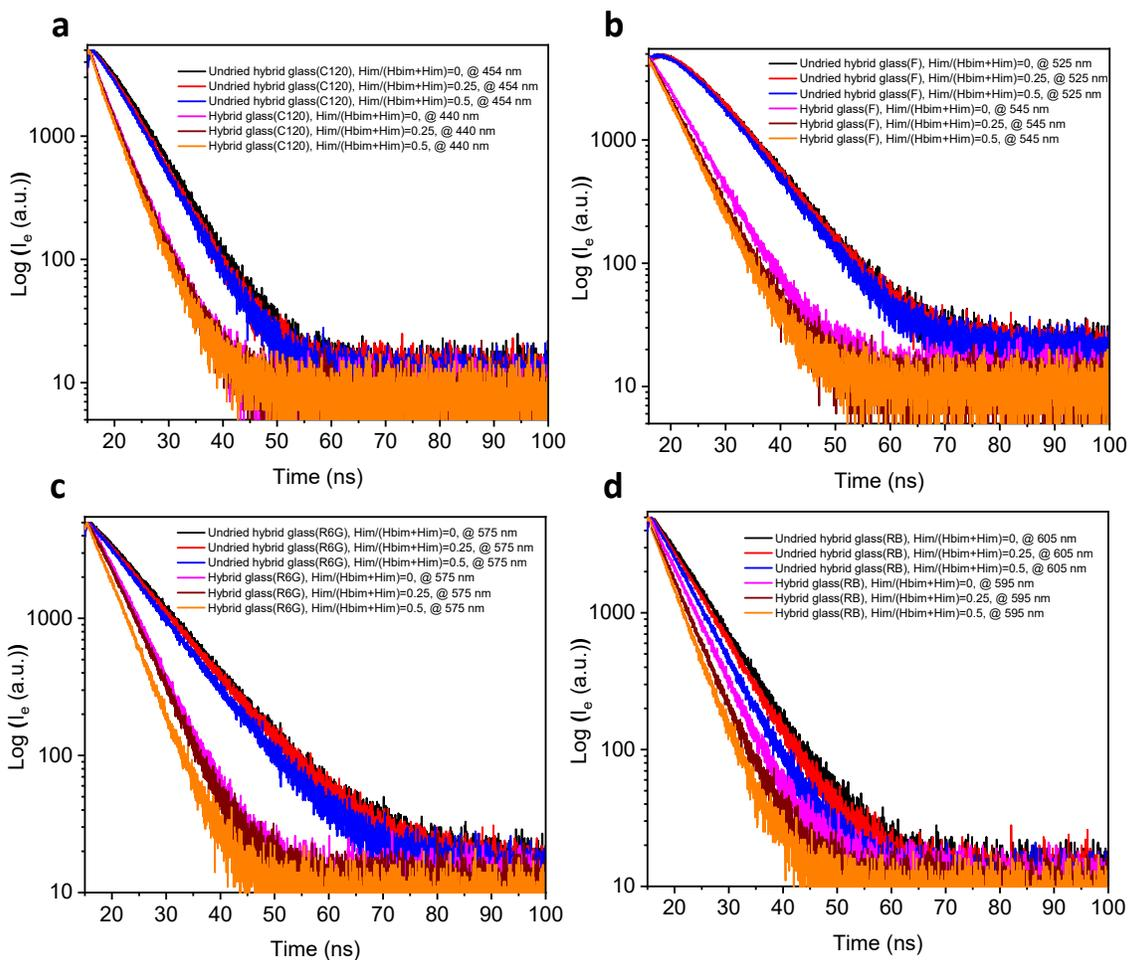
**Fig. S23.** PL decay curves of the undried hybrid glasses and hybrid glasses doped with **a**, C120, **b**, F, **c**, R6G, and **d**, RB at Him/(Hbim+Him) = 0, 0.25, and 0.5.
