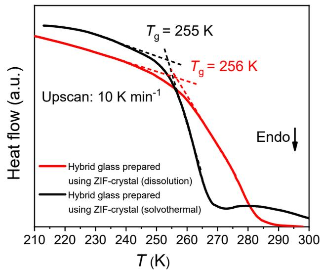
**Fig. S16.** DSC traces of the prepared hybrid glasses using ZIF-7-III crystals that prepared by solvothermal and dissolution-recrystallization methods at  $H_{im}/(H_{bim}+H_{im}) = 0$ .
