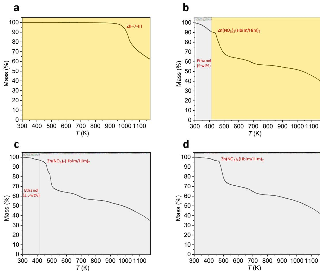
**Fig. S9.** TGA traces of the **a**, ZIF-7-III crystal, **b**, undried hybrid glass, **c**, hybrid glass, and **d**, brown hybrid glass at  $\text{Him}/(\text{Hbim}+\text{Him}) = 0.5$ .
