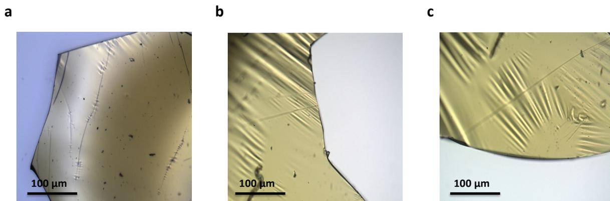
**Fig. S19.** Optical images of the brown hybrid glasses at **a**,  $H_{im}/(H_{bim}+H_{im}) = 0$ , **b**,  $H_{im}/(H_{bim}+H_{im}) = 0.25$ , and **c**,  $H_{im}/(H_{bim}+H_{im}) = 0.5$ .
