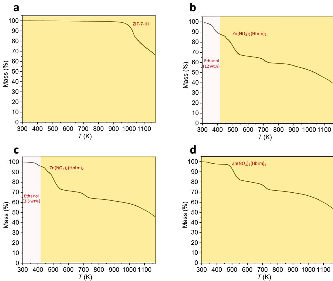
**Fig. S7.** TGA traces of the **a**, ZIF-7-III crystal, **b**, undried hybrid glass, **c**, hybrid glass, and **d**, brown hybrid glass at Him/(Hbim+Him) = 0.
