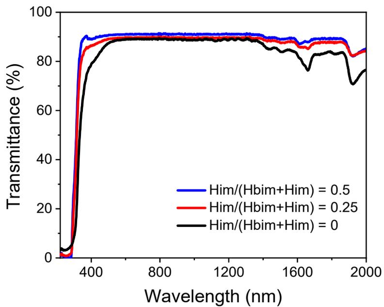
**Fig. S17.** UV-Vis-NIR transmission spectra of the hybrid glasses with a 1 mm in thickness at  $H_{im}/(H_{bim}+H_{im}) = 0$ , 0.25, and 0.5.
