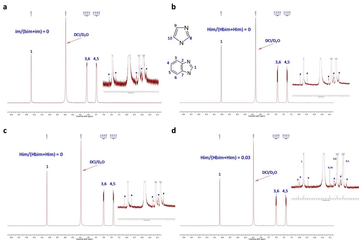
**Fig. S10.** Solution <sup>1</sup>H-NMR spectra of the **a**, ZIF-7-III crystal, **b**, undried hybrid glass, **c**, hybrid glass, and **d**, brown hybrid glass at Him/(Hbim+Him) = 0. The insets are the magnified <sup>1</sup>H-NMR spectra. The normalized proton integration values and the proton peak positions are in green and blue colors, respectively. The marked peaks with # are unknown. The insets are the molecular structures of Him and Hbim.
