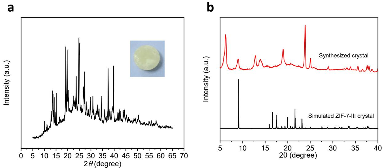
**Fig. S5.** PXRD patterns of the as-synthesized samples at  $\text{Him}/(\text{Hbim}+\text{Him}) = 0.75$  using **a**, network-solvation method and **b**, solvothermal method. The inset of **a** is a photograph of the corresponding sample.
