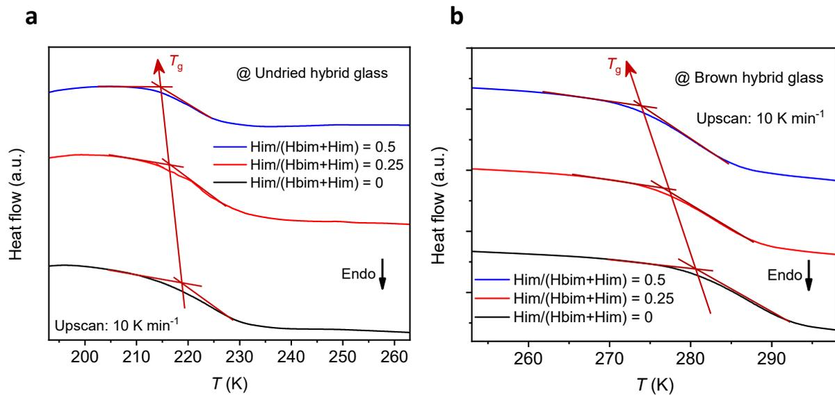
**Fig. S14.** DSC traces of the **a**, undried hybrid glasses and **b**, brown hybrid glasses at  $H_{im}/(H_{bim}+H_{im}) = 0, 0.25,$  and 0.5.
