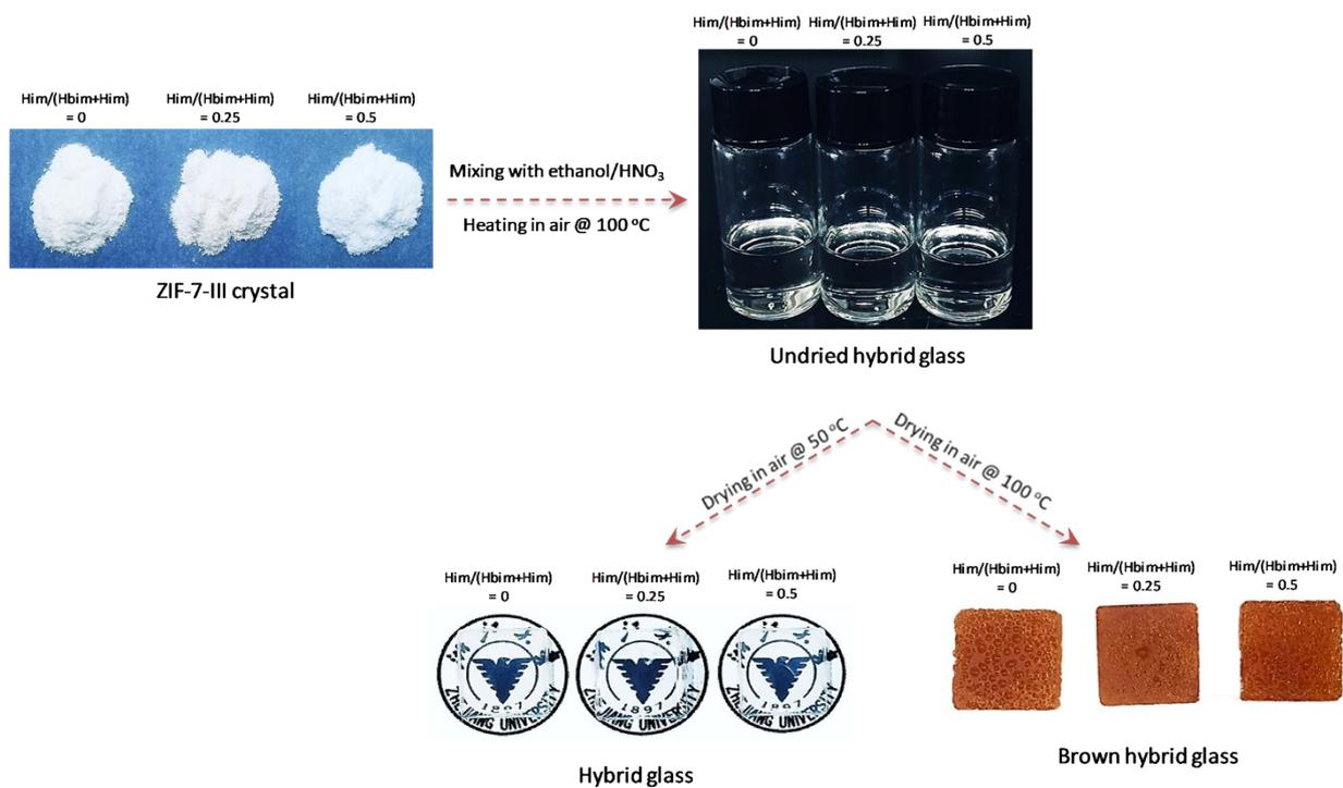
**Fig. S1.** Schematic illustration for the synthesis of the undried hybrid glasses, the hybrid glasses, and the brown hybrid glasses at  $\text{Him}/(\text{Hbim}+\text{Him}) = 0, 0.25, \text{ and } 0.5$ .
