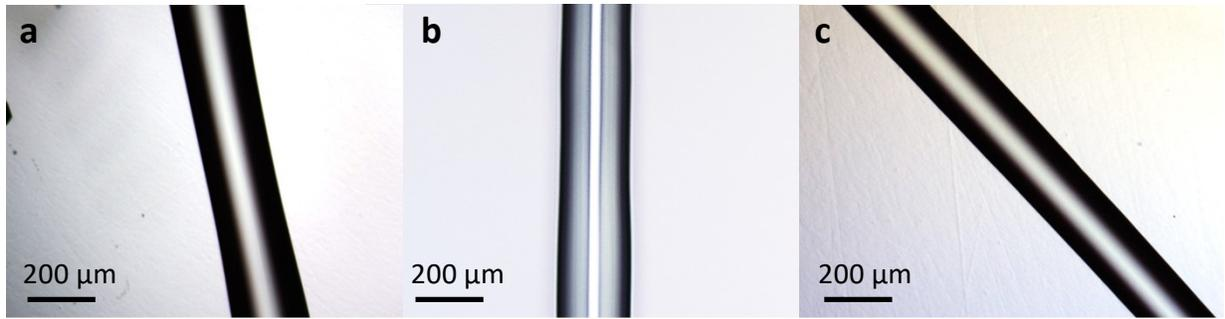
**Fig. S26.** Optical microscope images of the undoped hybrid glass fiber at **a**,  $\text{Him}/(\text{Hbim}+\text{Him}) = 0$ , **b**,  $\text{Him}/(\text{Hbim}+\text{Him}) = 0.25$ , and **c\text{Him}/(\text{Hbim}+\text{Him}) = 0.5.**
