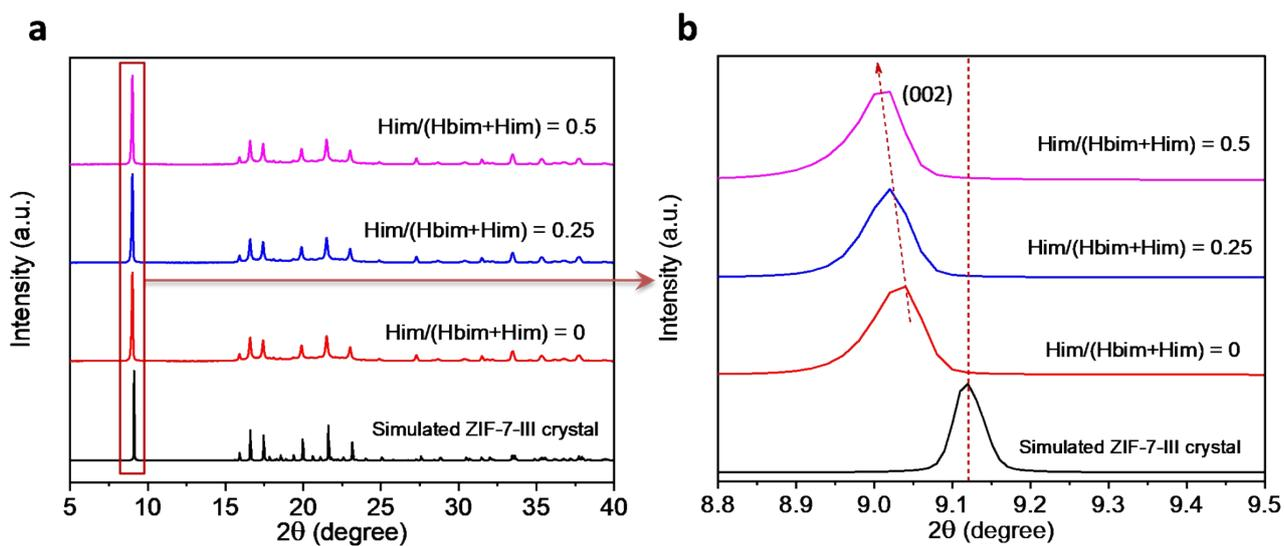
**Fig. S2. a**, PXRD patterns of the ZIF-7-III crystal at Him/(Hbim+Him) = 0, 0.25, and 0.5 synthesized by dissolution recrystallization method. **b**, The magnified pattern of (a) in the range of 8.8-9.5 degree. The observed peak shift in **b** is due to the increase of intermolecular spacing of ZIF-7-III crystal as a result of the substitution of Hbim by Him; where the molecular size of Him is smaller than that of Hbim.
