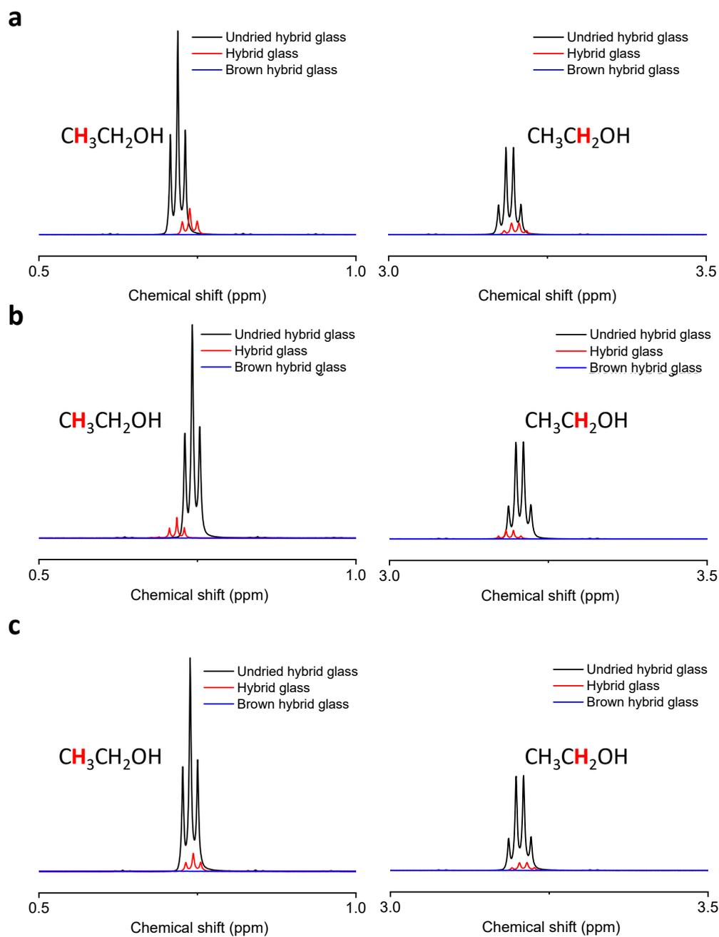
**Fig. S13.** Solution  $^1\text{H}$ -NMR spectra of the undried hybrid glasses, hybrid glasses, and brown hybrid glasses at **a**,  $\text{Him}/(\text{Hbim}+\text{Him}) = 0$ , **b**,  $\text{Him}/(\text{Hbim}+\text{Him}) = 0.25$ , and **c**,  $\text{Him}/(\text{Hbim}+\text{Him}) = 0.5$ .
