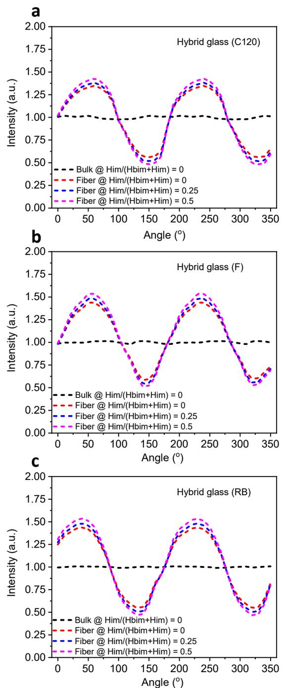
**Fig. S27.** The variation of integrated PL intensity with different polarization angles for the dried hybrid fiber and bulk glass doped with **a**, C120, **b**, F, and **c**, RB at  $H_{im}/(H_{bim}+H_{im}) = 0, 0.25,$  and  $0.5$ , under the excitation of polarized laser parallel to the fiber axis. The glass fibers doped with C120, F, and RB (a diameter of  $200\ \mu\text{m}$ ) and bulk glasses were excited by 405 nm and 460 nm polarized lasers, respectively.
