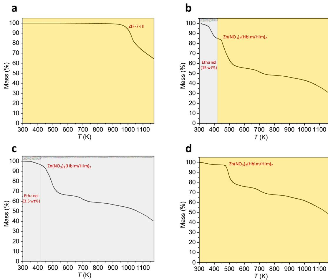
**Fig. S8.** TGA traces of the **a**, ZIF-7-III crystal, **b**, undried hybrid glass, **c**, hybrid glass, and **d**, brown hybrid glass at Him/(Hbim+Him) = 0.25.
