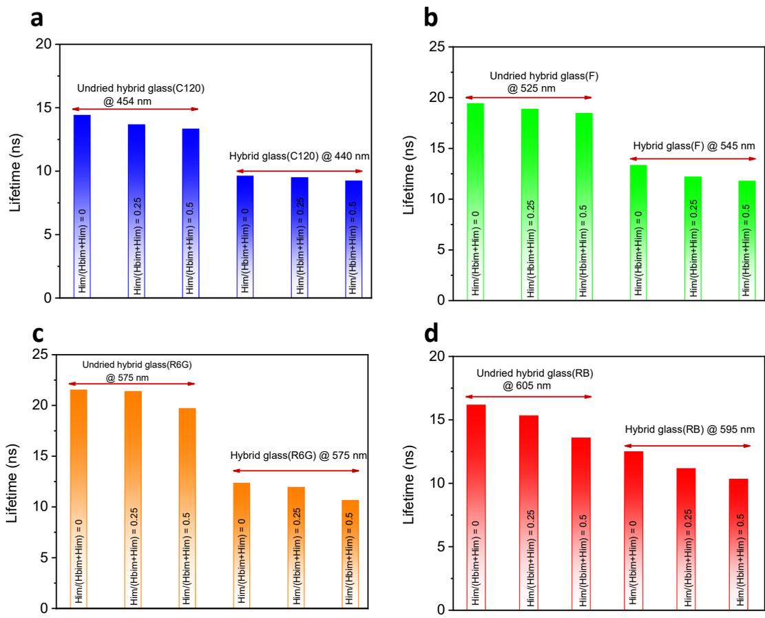
**Fig. S24.** Lifetime values of the undried hybrid glasses and hybrid glasses doped with **a**, C120, **b**, F, **c**, R6G, and **d**, RB at Him/(Hbim+Him) = 0, 0.25, and 0.5.
