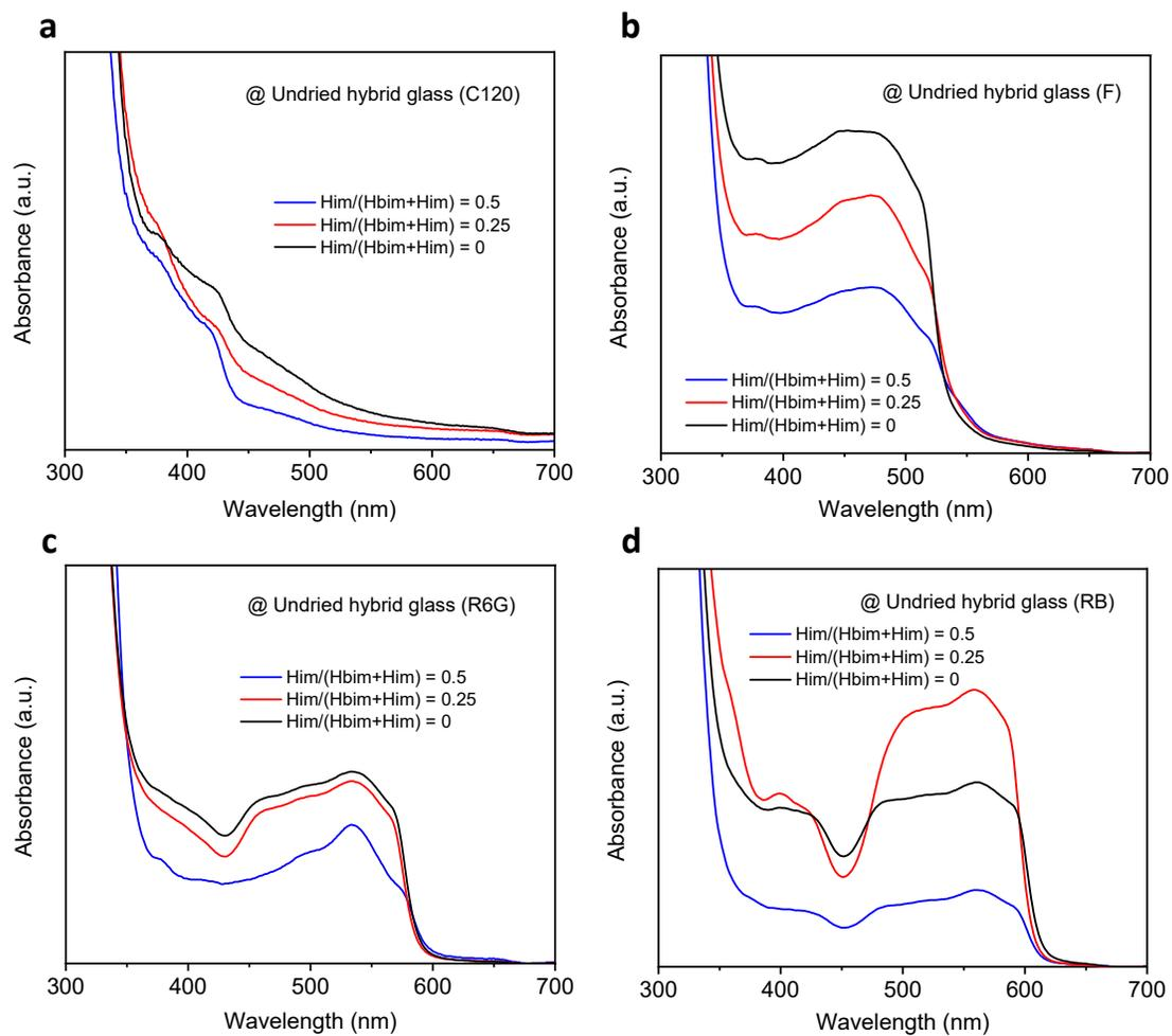
**Fig. S20.** UV-Vis absorption spectra of the undried hybrid glasses doped with **a**, C120, **b**, F, **c**, R6G, and **d**, RB at  $Him/(Hbim+Him) = 0, 0.25, \text{ and } 0.5$ .
