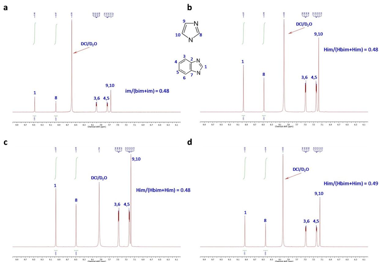
**Fig. S12.** Solution  $^1\text{H-NMR}$  spectra of the **a**, ZIF-7-III crystal, **b**, undried hybrid glass, **c**, hybrid glass, and **d**, brown hybrid glass at  $\text{Him}/(\text{Hbim}+\text{Him}) = 0.5$ . The normalized proton integration values and the proton peak positions are in green and blue colors, respectively. The insets are the molecular structures of Him and Hbim.
