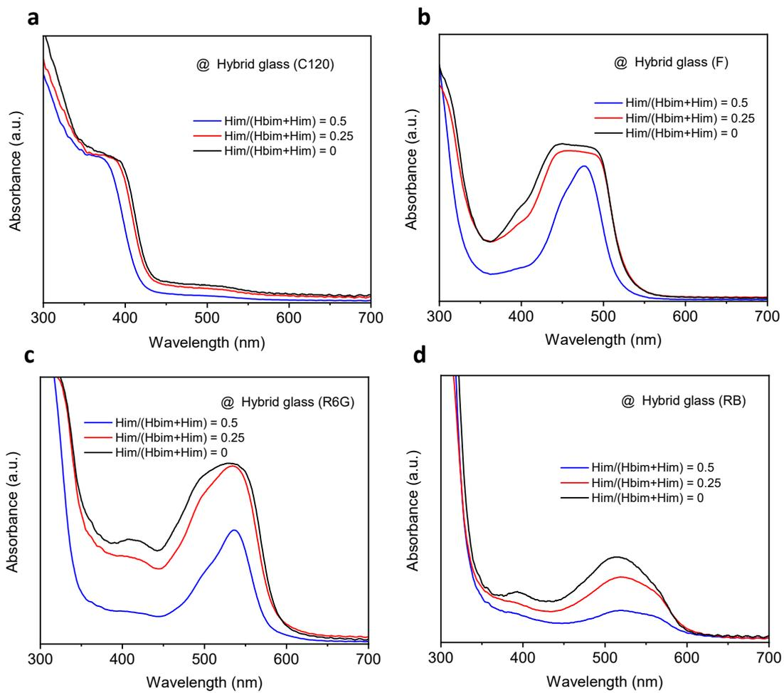
**Fig. S21.** UV-Vis absorption spectra of the hybrid glasses doped with **a**, C120, **b**, F, **c**, R6G, and **d**, RB at  $H_{im}/(H_{bim}+H_{im}) = 0, 0.25, \text{ and } 0.5$ .
