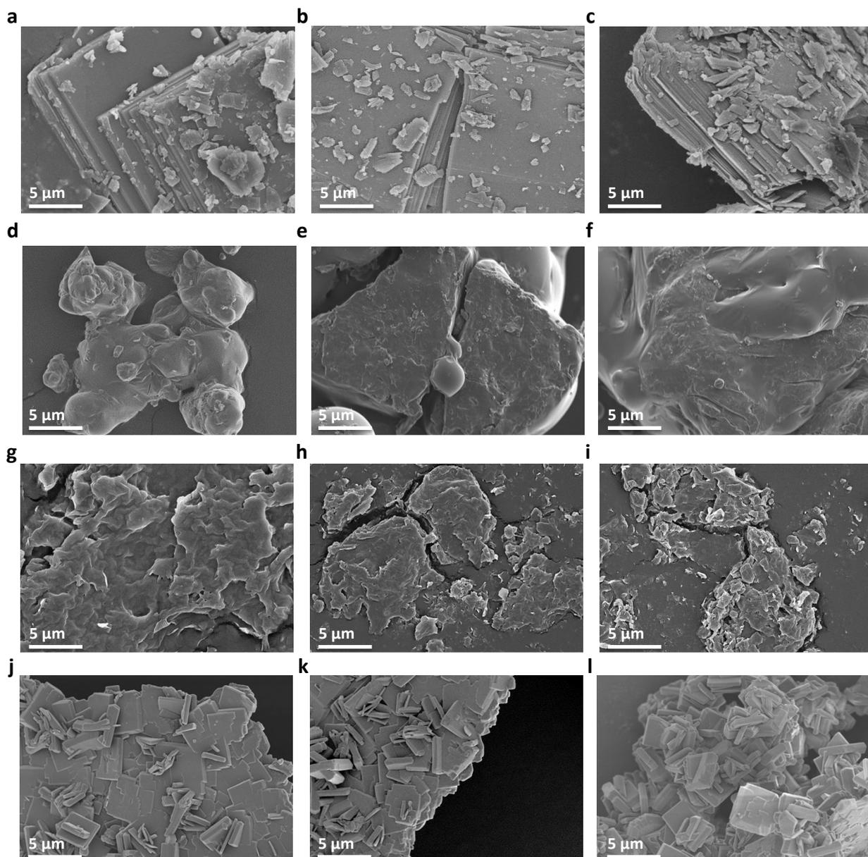
**Fig. S6.** SEM images of the **a-c**, ZIF-7-III crystals (solvothermal), **d-f**, hybrid glasses (solvation), **g-i**, brown hybrid glasses, and **j-l**, ZIF-7-III crystals (dissolution) at **a, d, g, j**,  $\text{Him}/(\text{Hbim}+\text{Him}) = 0$ , **b, e, h, k**,  $\text{Him}/(\text{Hbim}+\text{Him}) = 0.25$ , and **c, f, i, l**,  $\text{Him}/(\text{Hbim}+\text{Him}) = 0.5$ .
