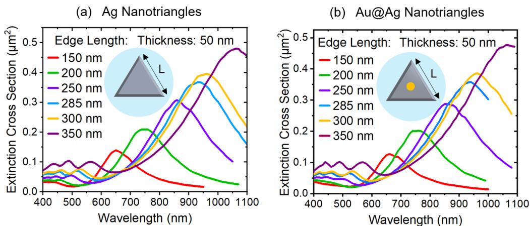
**Figure S11.** Simulations showing a comparison of the extinction spectra for (a) pure Ag nanotriangles and (b) Ag nanotriangles containing a centrally located Au seed (diameter = 75 nm) as the nanotriangle edge length is varied from 150 to 350 nm. It should be noted that the two structures show a near-identical response. Simulations include a 20 nm thick sapphire substrate.
