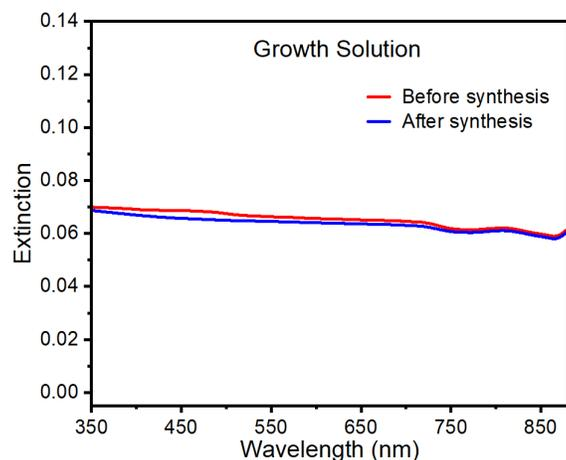
**Figure S2.** Extinction spectra of the growth solution taken before and after a substrate-based Ag nanotriangle synthesis. The fact that the two spectra overlap and appear featureless indicates that a measurable Ag colloid is unable to form over the 20 min duration of the synthesis.
