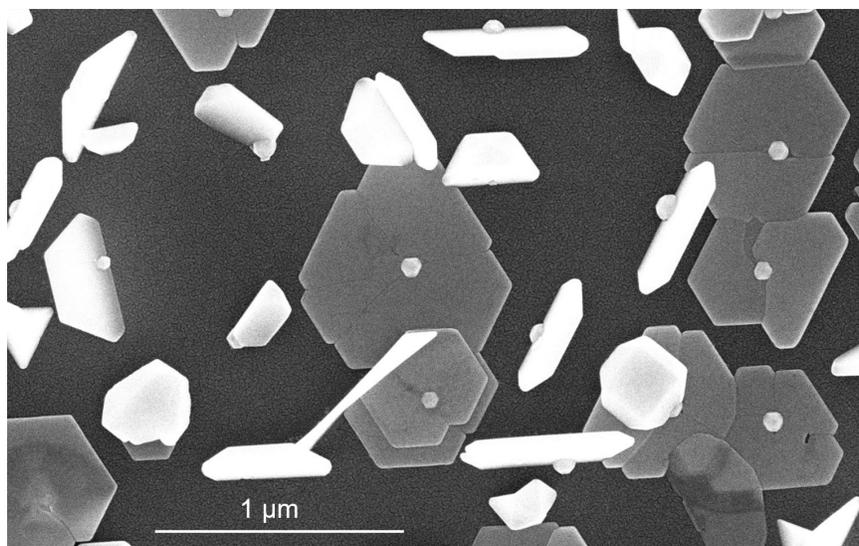
**Figure S1.** SEM image of Ag nanoplates derived from periodic arrays of Ag seeds. Ag seeds proved unsatisfactory in that they yielded a high percentage of structures with growth trajectories that are away from the surface of the substrate. When in-plane growth occurs, the seeds show a strong tendency toward three-dimensional growth such that the final product appears as a nanoplate from which a larger central structure protrudes.
