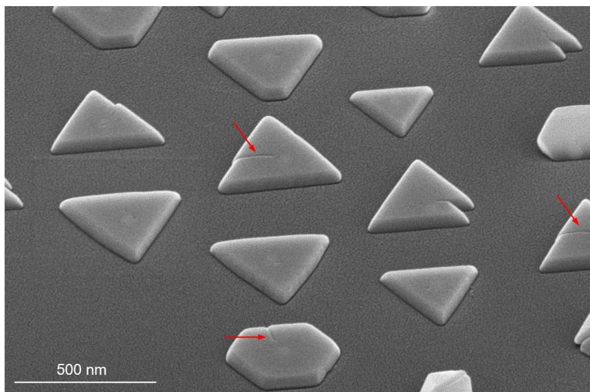
**Figure S6.** High-resolution SEM images showing the crack-like features exhibited by many of the Ag nanoplates.
