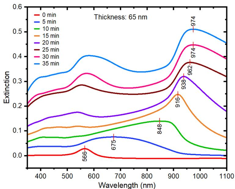
**Figure S10.** Time-dependent extinction spectra for a Ag nanotriangle synthesis that originates from Au seeds with a thickness of 65 nm.
