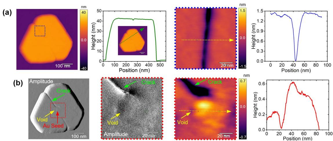
**Figure S9.** AFM characterization of a hexagonal nanoplate showing (a) crack- and (b) void-like features. It should be noted that the observed features are analogous to those observed for triangular nanoplates (Figure 5).
