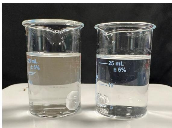
**Figure S3.** Image of the Ag nanoplate growth solution taken after a 20 min synthesis where acetonitrile is excluded from the synthesis (left) and included in the synthesis (right). The data confirms that acetonitrile is needed to suppress the homogeneous nucleation of Ag nanoparticles within the growth solution.
