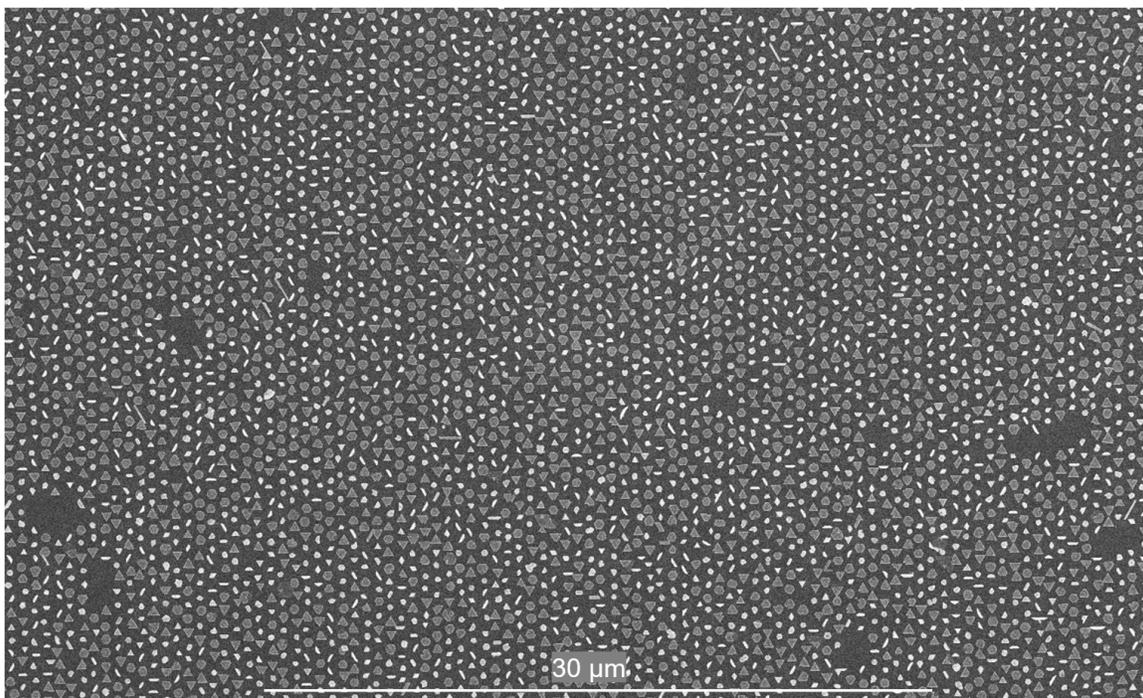
**Figure S4.** SEM image of the Ag nanoplate array taken at low magnification. It should be noted that array positions lacking structures are caused by damage to the nanoimprint lithography stamp.
