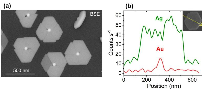
**Figure S7.** (a) BSE SEM image of hexagonal plates where Au seeds are clearly visible. (b) Line scan for a hexagonal plate showing a Au seed positioned in the middle of the Ag nanoplate.
