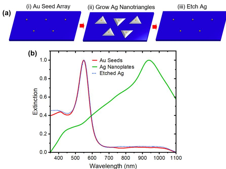
**Figure S8.** (a) Schematic and (b) the associated normalized extinction spectra taken for the same Au seed array (i) before being placed into the Ag nanotriangle growth solution, (ii) after the Ag nanoplate growth, and (iii) after the removal of the Ag with an etchant. The fact that the Au plasmon is near-identical for (i) and (iii) provides evidence that Au–Ag interdiffusion at the interface is minimal during the synthesis.
