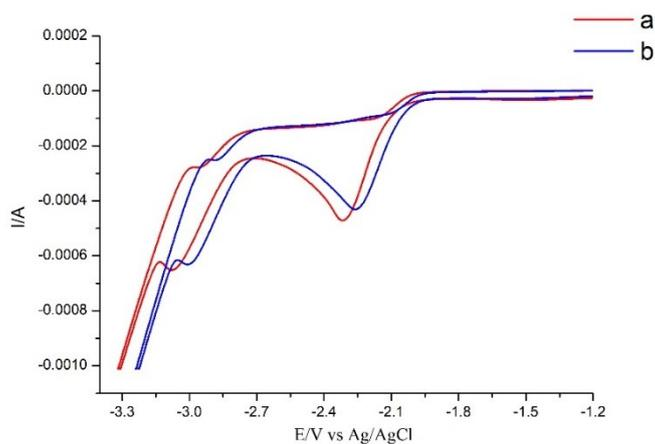
**Figure S2-5** Cyclic voltammograms in DMF + 0.1 M  $n\text{Bu}_4\text{NBF}_4$ . a) **1a** (0.2 mmol),  $E_{p/2} = -2.31$  V,  $i_{p,c} = -5.0$  mA. b) **1a** (0.2 mmol) and Fullerene-C60 (0.2 mmol),  $E_{p/2} = -2.33$  V,  $i_{p,c} = -5.3$  mA.
