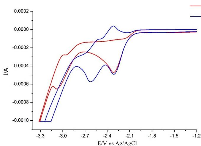
**Figure S2-2** Cyclic voltammograms in DMF + 0.1 M  $n\text{Bu}_4\text{NBF}_4$ . a) **1a** (0.2 mmol),  $E_{p/2} = -2.31$  V,  $i_{p,c} = -5.0$  mA. b) **1a** (0.2 mmol) and Anthracene (0.2 mmol),  $E_{p/2} = -2.31$  V,  $i_{p,c} = -5.1$  mA.
