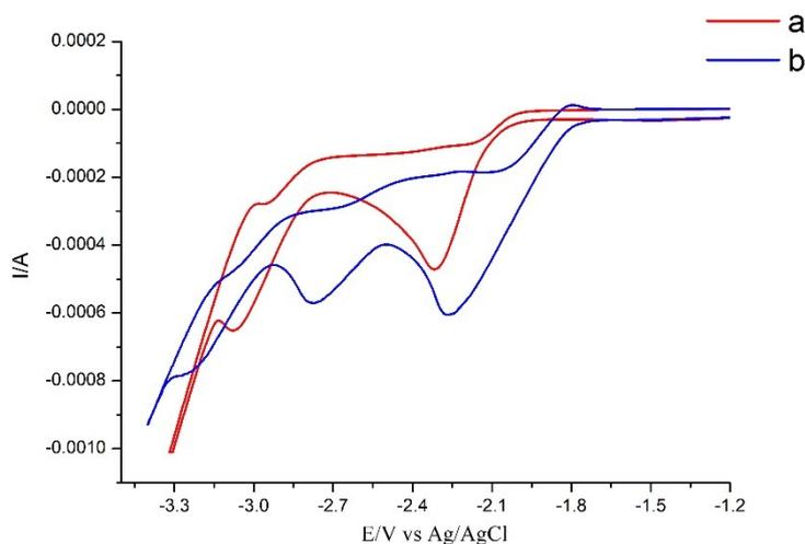
**Figure S2-1** Cyclic voltammograms in DMF + 0.1 M  $n\text{Bu}_4\text{NBF}_4$ . a) **1a** (0.2 mmol),  $E_{p/2} = -2.31$  V,  $i_{p,c} = -5.0$  mA. b) **1a** (0.2 mmol) and Phenanthrene (0.2 mmol),  $E_{p/2} = -2.25$  V,  $i_{p,c} = -6.3$  mA.
