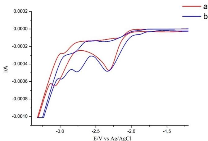
**Figure S2-4** Cyclic voltammograms in DMF + 0.1 M  $n\text{Bu}_4\text{NBF}_4$ . a) **1a** (0.2 mmol),  $E_{p/2} = 2.31$  V,  $i_{p,c} = -5.0$  mA. b) **1a** (0.2 mmol) and Fluorene (0.2 mmol),  $E_{p/2} = -2.33$  V,  $i_{p,c} = -5.1$  mA.
