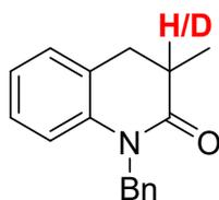
1-benzyl-3,3-dimethyl-3,4-dihydroquinolin-2(1H)-one (**2a** & **2a-d**), Colorless oily. Petroleum ether/ethyl acetate = 20/1-10/1 (v/v) as eluent for column chromatography <sup>1</sup>H NMR (400 MHz, Chloroform-*d*) δ 7.32 – 7.28 (m, 2H), 7.24 – 7.20 (m, 4H), 7.13 – 7.09 (m, 1H), 7.03 – 6.99 m, 1H), 6.89 (dd, *J* = 8.1, 0.9 Hz, 1H), 5.26 – 5.14 (m, 2H), 2.88 (dd, *J* = 15.6, 4.8 Hz, 1H), 2.65 – 2.56 (m, 1H), 1.33 (d, *J* = 7.4 Hz, 3H).
