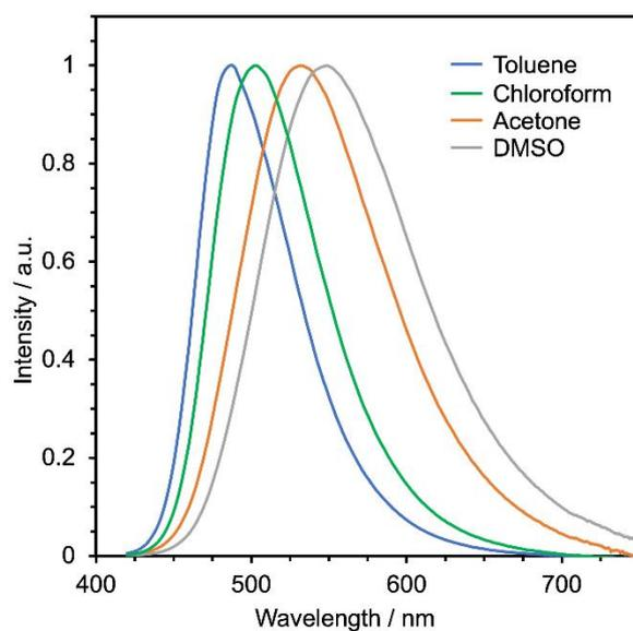
Figure S5. Emission spectra of **TANaph 3** in various solvents ( $1.0 \times 10^{-5}$  M).
