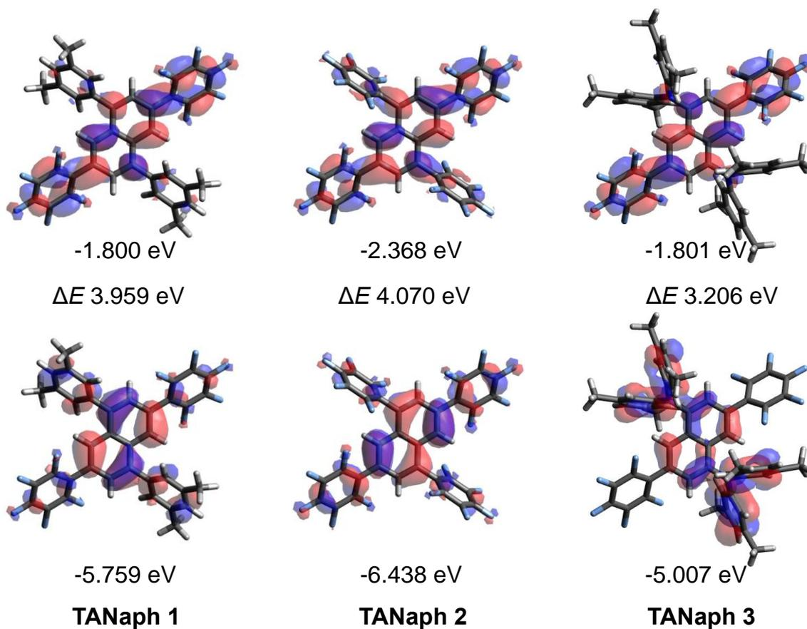
Figure S3. Calculated HOMO distribution (bottom), LUMO distribution (top), and the bandgap of TANaphs (DFT: B3LYP/6-31(G)).
