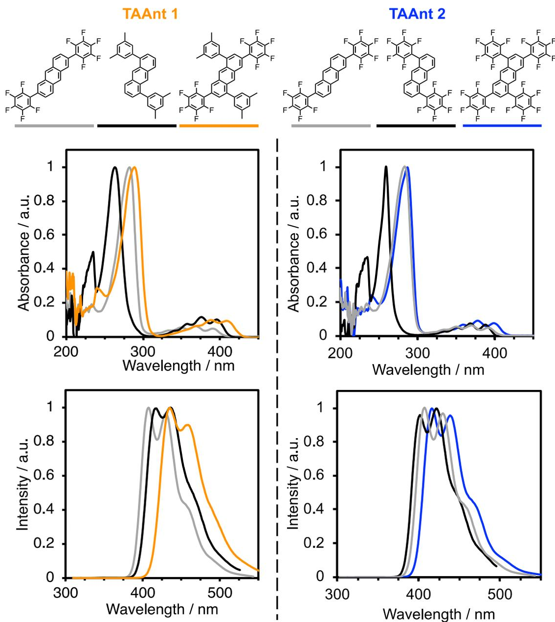
Figure S7. Comparison UV-vis absorption (top) and emission spectra (bottom) of TAAnts and the partial structure compounds in chloroform solution ( $1.0 \times 10^{-5}$  M).<sup>2,3</sup>
