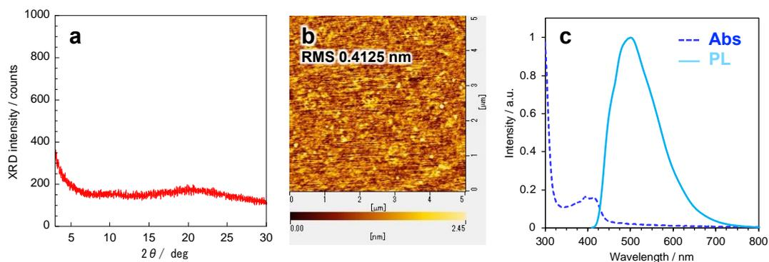
Figure S8. (a) XRD spectrum, (b) AFM image, and (c) UV-vis absorption (dotted line) and emission spectra (solid line) of **TAAnt 1** in the film state.
