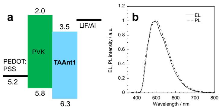
Figure S11. (a) The OLED structure and (b) EL and PL spectra.
