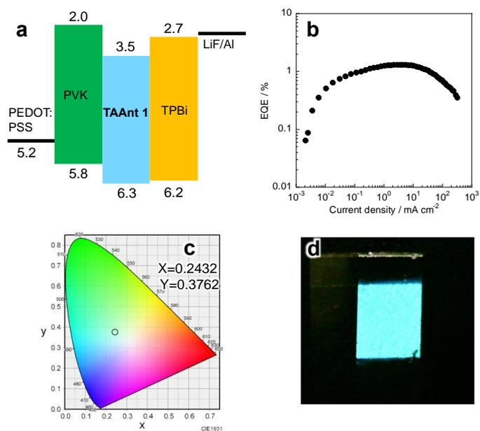
Figure S10. (a) The OLED structure, (b) EQE–current density characteristics, (c) CIE chromaticity coordinates, and (d) Photograph of OLED luminescence.
