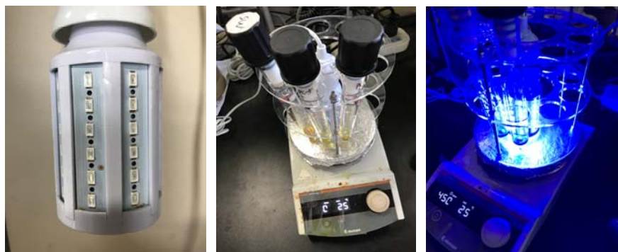
Figure S1 Photoreactor used in this work (20 W blue LEDs, \lambda_{\text{max}} = 454 nm).
