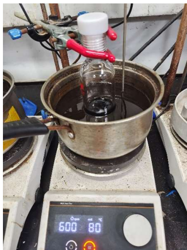
Figure S2 | The heat source used in the gram scale reaction.
