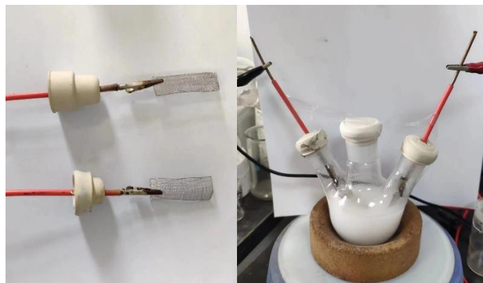
Fig. S23. Gram electrolysis device (platinum mesh: length 5.0 cm, width 2.0 cm, immersion depth 2.0 cm)
