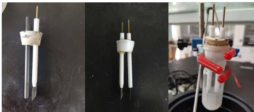
Fig. S22. Electrolysis setup (graphite rod: diameter 0.6 cm, length 10 cm; platinum plate: 1.5 cm *1.5 cm)
