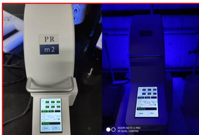
43 *Figure S1: The Blue LED Photoreactor set-up used.*
