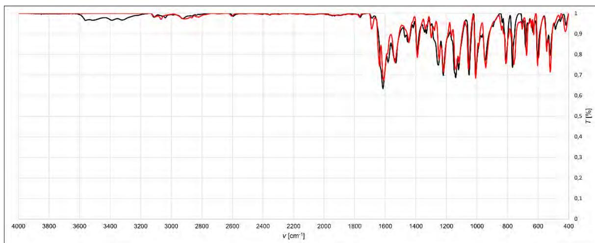
**Figure S59.** IR spectrum after grinding equal amounts of DMAP and XB complex **3a** under neat conditions for 2 min (red) and comparison with the IR spectrum of symmetric iodine(I) complex **4a** obtained from solution (black).
