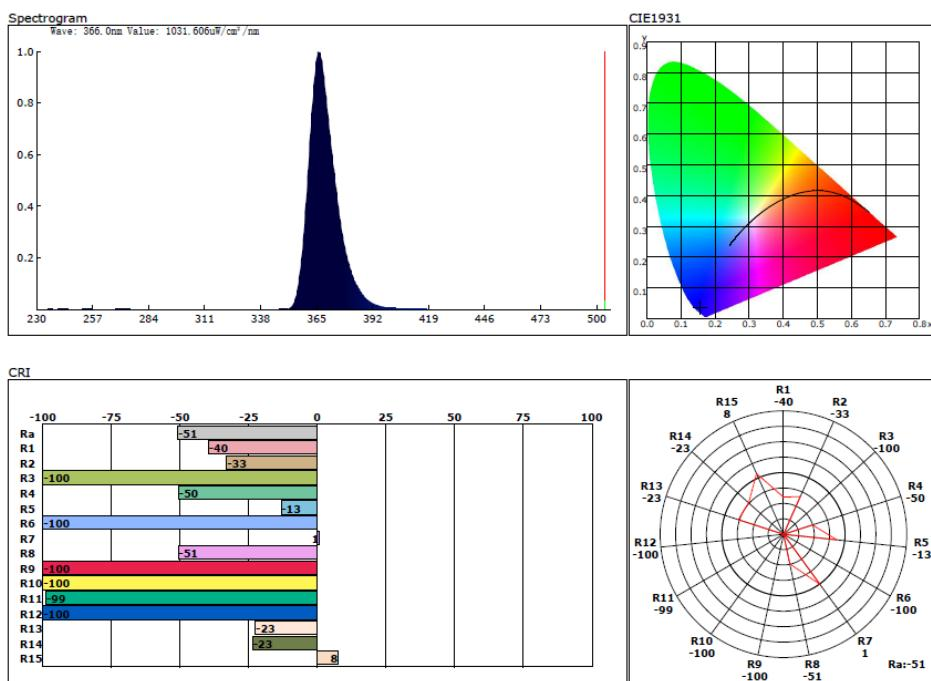
**Figure S1.** The emission spectra and spectral distribution of the purple LEDs
