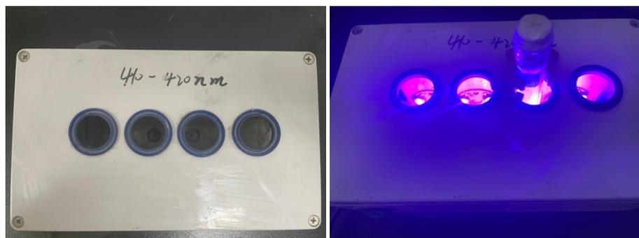
We use a commercially available 24 W 410-420 nm purple LED lamp as the reaction light source. At ambient temperature, the sample is placed approximately 2 cm away from the lamp. The material of the irradiation vessel is quartz. We also measured the wavelength of the LED light by ourselves (recorded on an AVANTES® AvaSpec-ULS2048 spectrometer instrument). The result was shown as follow:
