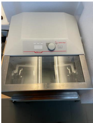
Fig. S1. Anton Paar BM500 used in this study. Fig. S2. Stainless-steel jar used in this study.
