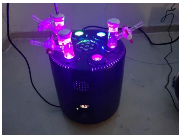
Figure S1. Photo of the reaction set-up ( \lambda = 410\text{--}415\text{ nm} ).
