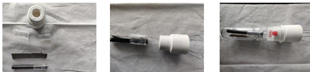
Figure S2. Left: Materials for making the electrodes; Middle: The assembled electrodes; Right: The assembled electrolytic cell.
