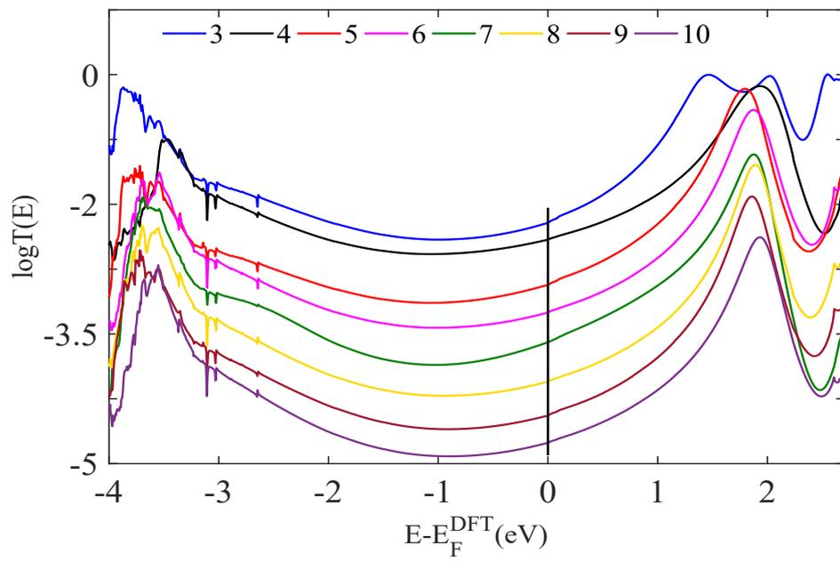
**Supplementary Figure 5.** Transmission coefficient curves of alkane chains with (*Au-SMe*), for  $n=3$  to 10, carbon atoms of linear chains against electron energy  $E$ .
