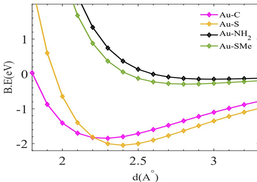
**Supplementary Figure 2.** Binding energy of alkane linear chains to gold as a function of molecule-contact distance. The equilibrium distance (i.e. the minimum of the binding energy curve) is found to be approximately 2.3, 2.4, 2.8 and 3.0 Å, for  $Au-C$ ,  $Au-S$ ,  $Au-NH_2$  and  $Au-SMe$  (top to bottom).
