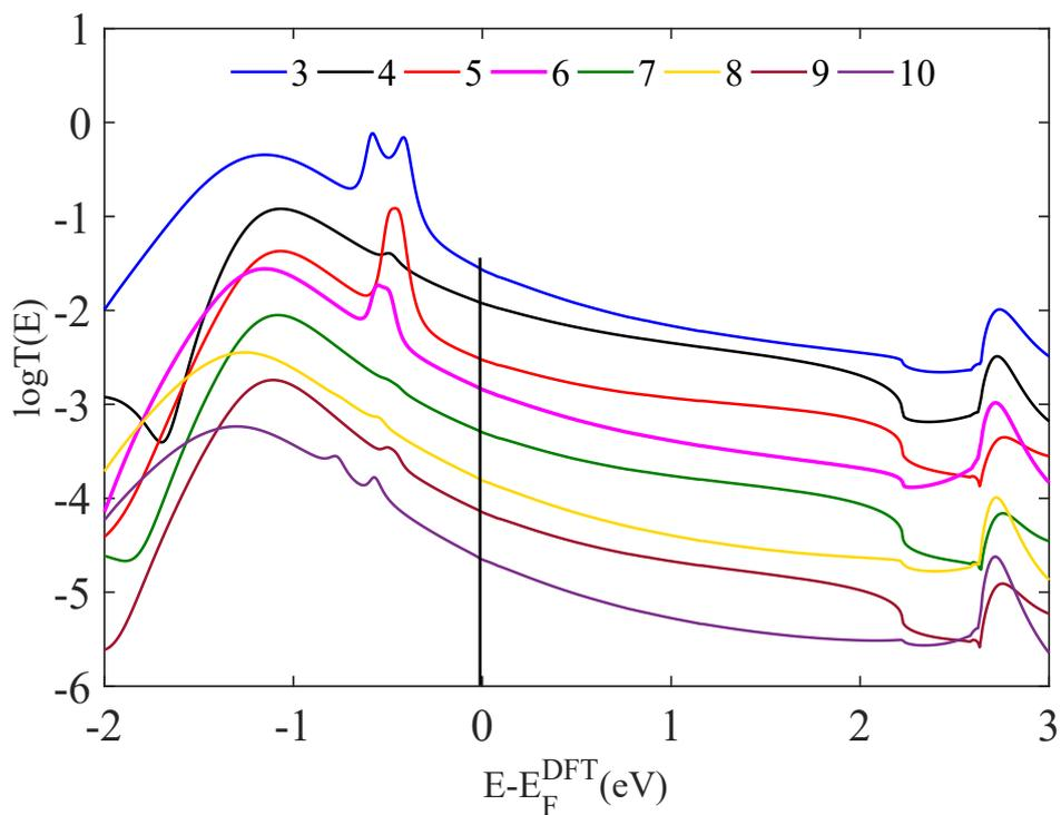
**Supplementary Figure 6.** Transmission coefficients of alkanes chains with (*Au-S*), for  $n=3$  to 10, carbon atoms of linear chains against electron energy  $E$ .
