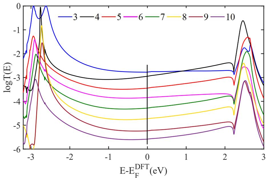
**Supplementary Figure 4.** Transmission coefficient curves of alkane chains with (*Au-Amine*), for  $n=3$  to 10, carbon atoms of linear chains against electron energy  $E$ .
