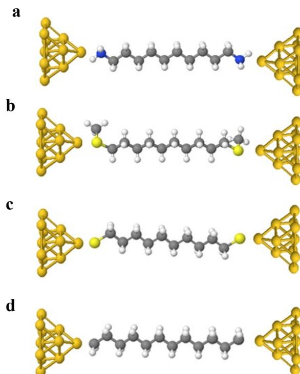
**Supplementary Figure 3.** Examples of fully relaxed alkane derivatives in Au|alkane chains|Au junctions: (a), (b), (c) and (d):  $n = 10$  linear chains connected to gold electrodes via amine, thiomethyl, thiol and direct carbon anchor groups respectively (for clarity only 1 chain out of 8 are shown for each terminal group).
