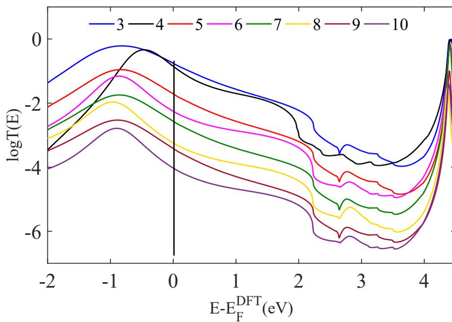
**Supplementary Figure 7.** Transmission coefficients of alkanes chains with (*Au-C*), for  $n=3$  to 10, carbon atoms of linear chains against electron energy  $E$ .
