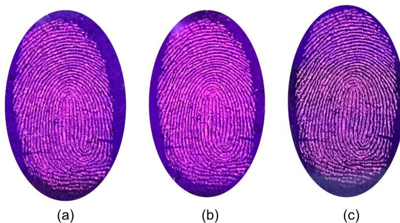
Fig. S14 Long-term stability image of Eu-MOF developed LFPs after storage for (a) 0 day, (b) 7 days, and (c) 30 days.
