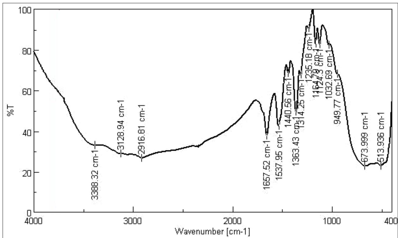
Figure S35: FTIR spectrum of compound HB-3 over TiO<sub>2</sub>.
