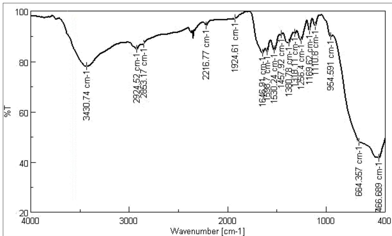
Figure S40: FTIR spectrum of compound HB-8 over TiO<sub>2</sub>.
