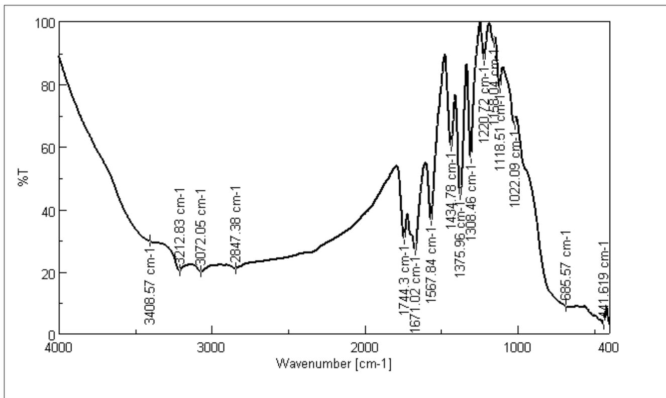
Figure S34: FTIR spectrum of compound HB-2 over TiO<sub>2</sub>.
