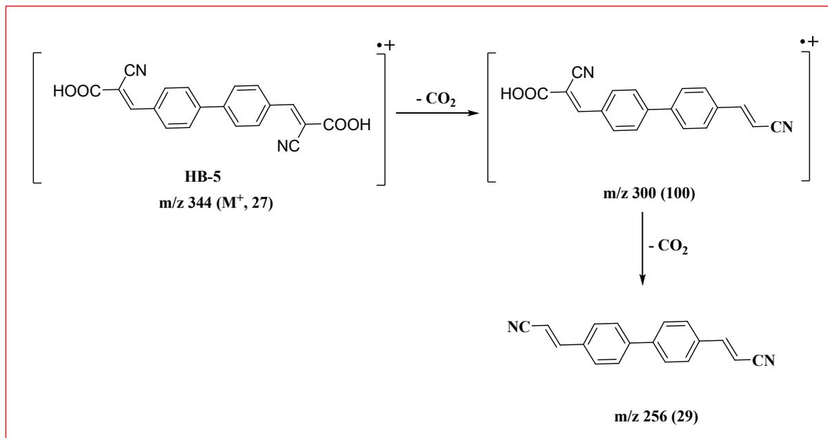
**Figure S20:** Mass fragmentation pattern of biphenyl dye **HB-5**.
