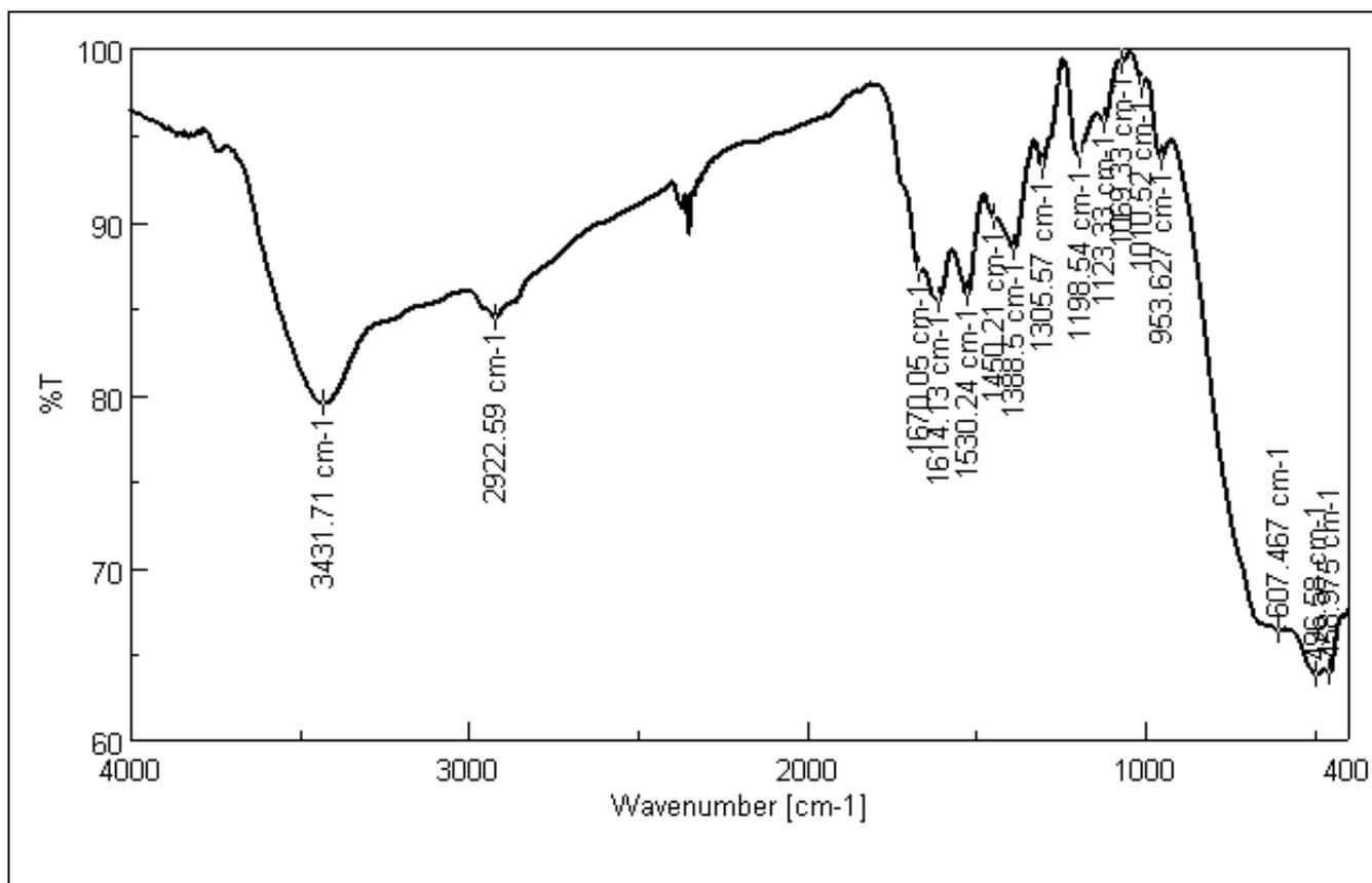
Figure S39: FTIR spectrum of compound HB-7 over TiO<sub>2</sub>.
