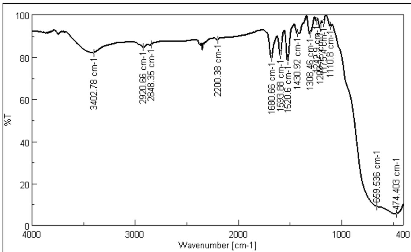
**Figure S36: FTIR spectrum of compound HB-4 over TiO<sub>2</sub>.**
