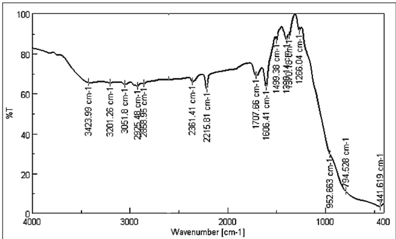
Figure S37: FTIR spectrum of compound HB-5 over TiO<sub>2</sub>.
