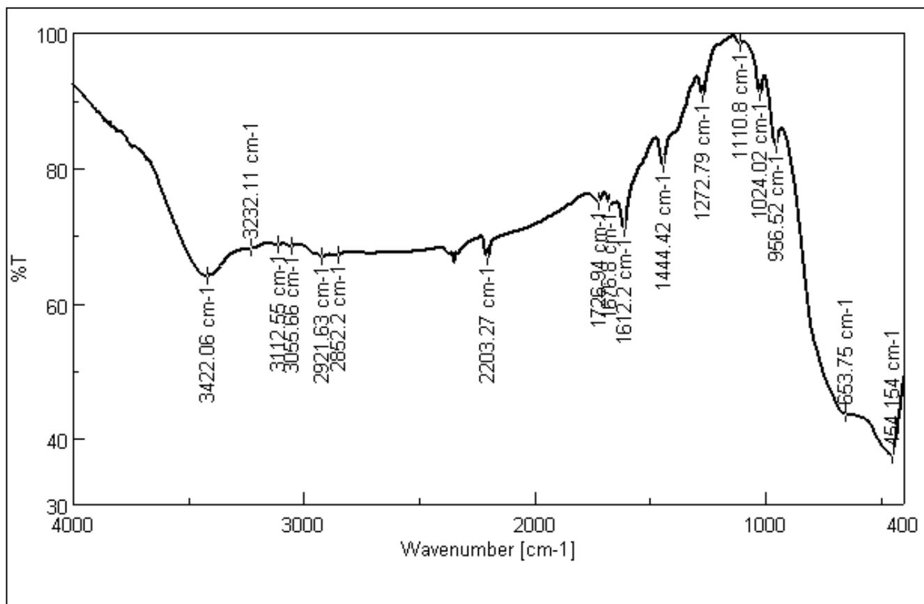
Figure S33: FTIR spectrum of compound HB-1 over TiO<sub>2</sub>.
