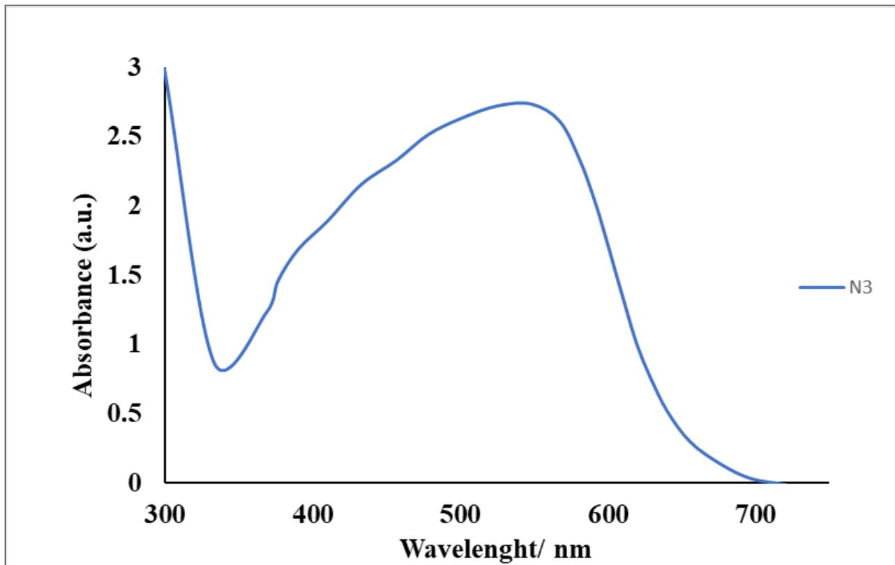
Fig. (S31): UV-Vis. absorption of N3 on TiO<sub>2</sub>.
