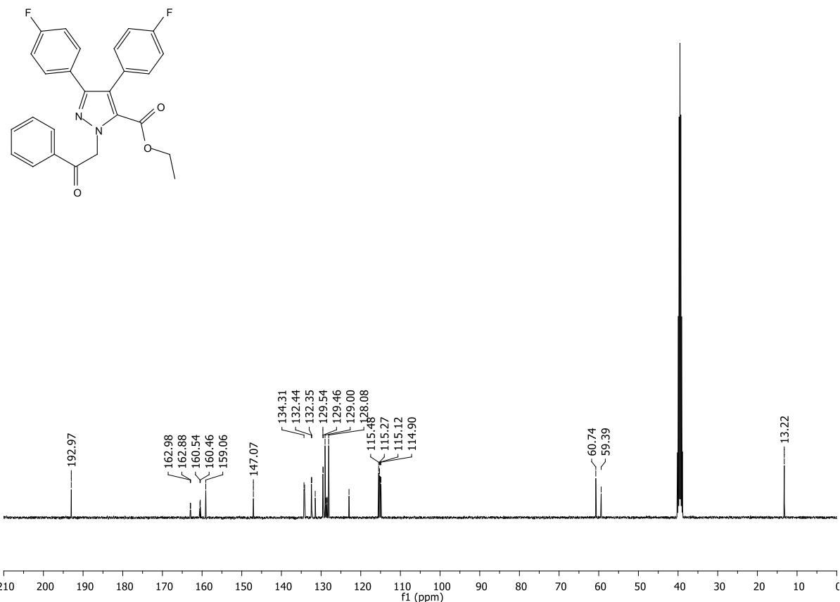
**Figure S97.** <sup>13</sup>C NMR spectrum (101 MHz, DMSO-*d*<sub>6</sub>) of ethyl 3,4-bis(4-fluorophenyl)-1-(2-oxo-2-phenylethyl)-1*H*-pyrazole-5-carboxylate (**6k**).
