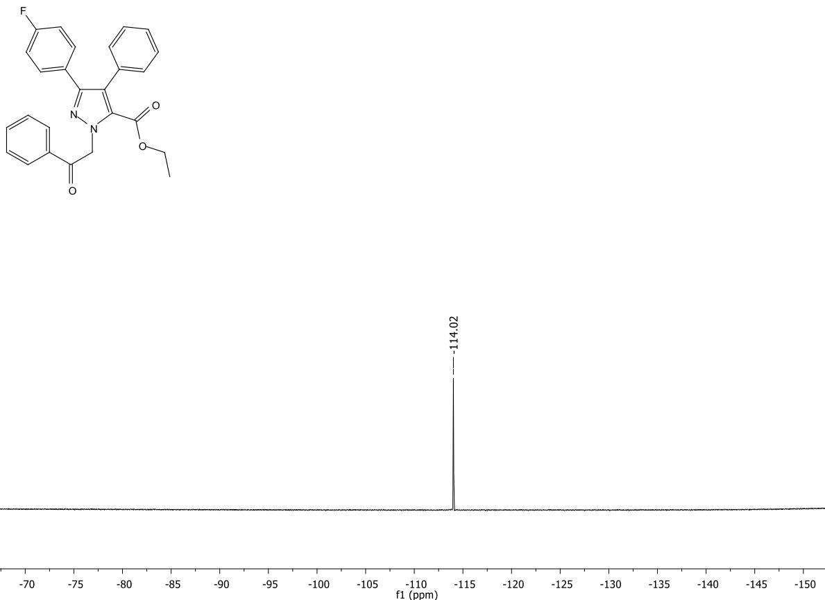
**Figure S94.**  $^{19}\text{F}$  NMR spectrum (376 MHz,  $\text{DMSO}-d_6$ ) of ethyl 3-(4-fluorophenyl)-1-(2-oxo-2-phenylethyl)-4-phenyl-1*H*-pyrazole-5-carboxylate (**6j**).
