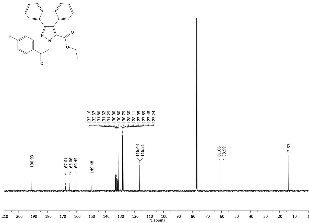
**Figure S62.**  $^{13}\text{C}$  NMR spectrum (101 MHz,  $\text{CDCl}_3$ ) of ethyl 1-[2-(4-fluorophenyl)-2-oxoethyl]-3,4-diphenyl-1*H*-pyrazole-5-carboxylate (**6c**).
