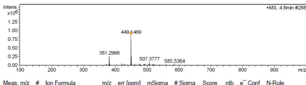
**Figure S73.** HRMS (ESI-TOF) spectrum of ethyl 1-[2-(4-hydroxyphenyl]-2-oxoethyl)-3,4-diphenyl-1*H*-pyrazole-5-carboxylate (**6e**).
