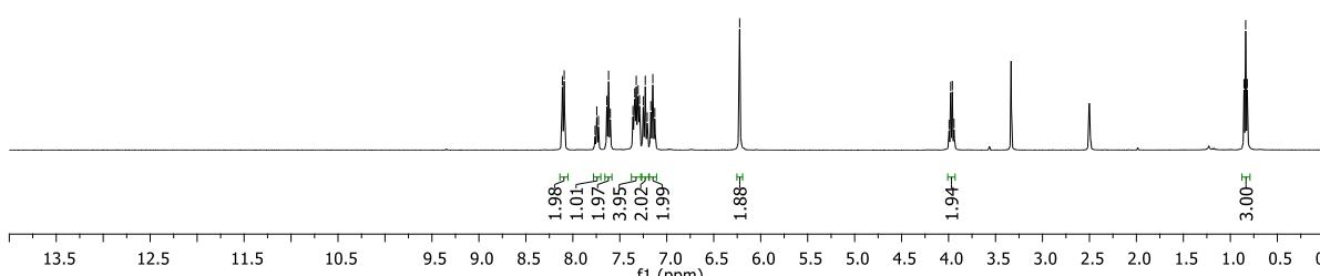
**Figure S96.** <sup>1</sup>H NMR spectrum (400 MHz, DMSO-d<sub>6</sub>) of ethyl 3,4-bis(4-fluorophenyl)-1-(2-oxo-2-phenylethyl)-1*H*-pyrazole-5-carboxylate (**6k**).
