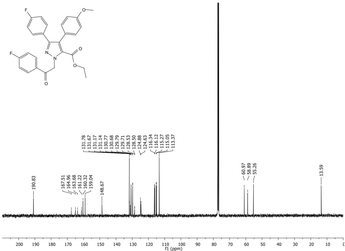
**Figure S112.**  $^{13}\text{C}$  NMR spectrum (101 MHz,  $\text{CDCl}_3$ ) of ethyl 3-(4-fluorophenyl)-1-[2-(4-fluorophenyl)-2-oxoethyl]-4-(4-methoxyphenyl)-1*H*-pyrazole-5-carboxylate (**6n**).
