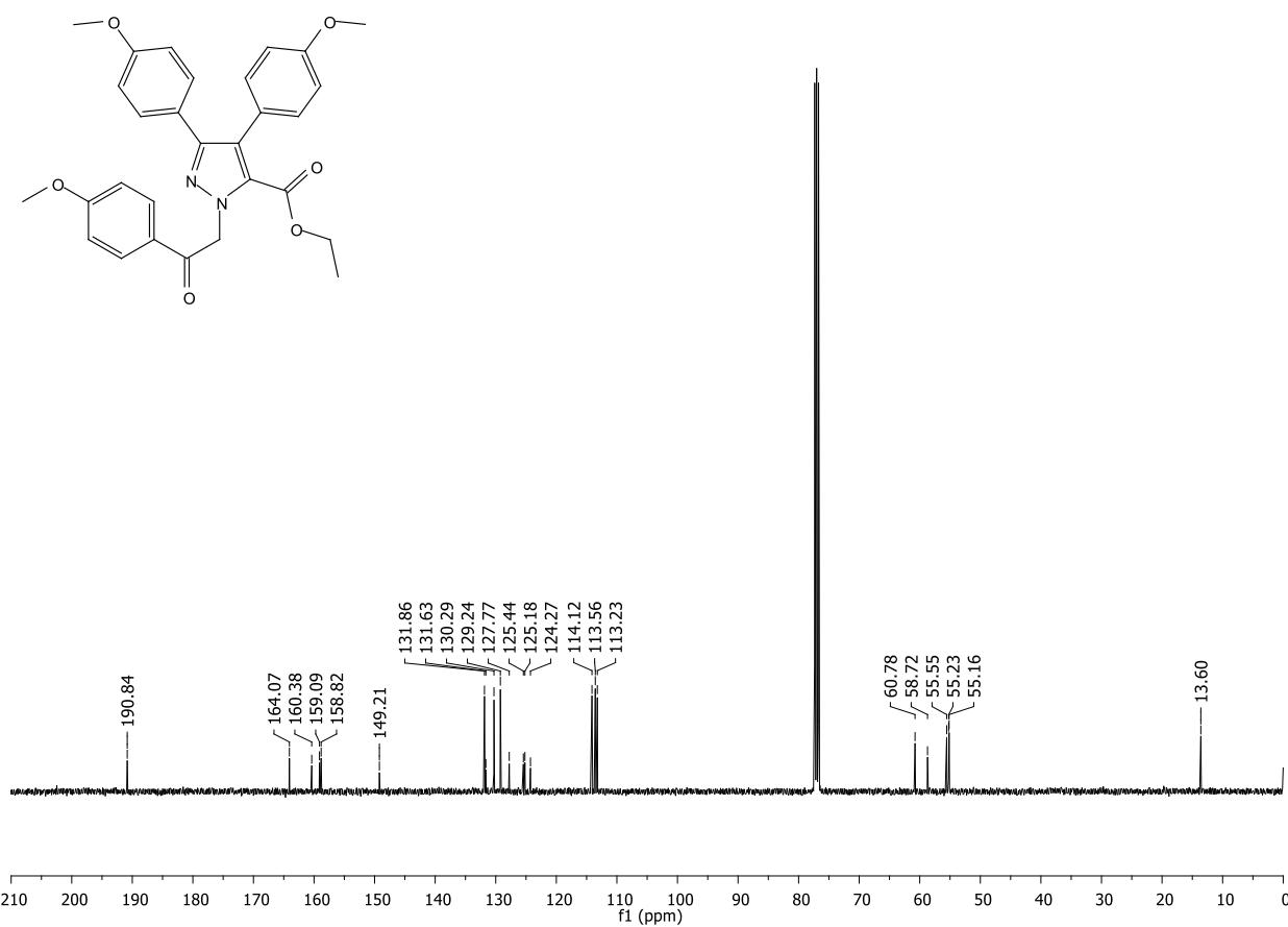
**Figure S79.**  $^{13}\text{C}$  NMR spectrum (101 MHz,  $\text{CDCl}_3$ ) of ethyl 3,4-bis(4-methoxyphenyl)-1-[2-(4-methoxyphenyl)-2-oxoethyl]-1*H*-pyrazole-5-carboxylate (**6g**).
