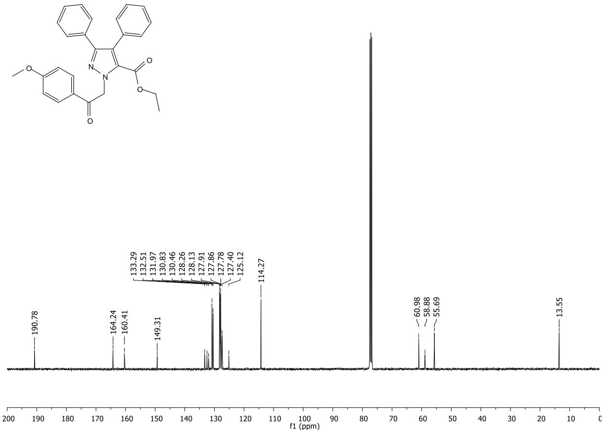
**Figure S58.**  $^{13}\text{C}$  NMR spectrum (101 MHz,  $\text{CDCl}_3$ ) of ethyl 1-[2-(4-methoxyphenyl)-2-oxoethyl]-3,4-diphenyl-1*H*-pyrazole-5-carboxylate (**6b**).
