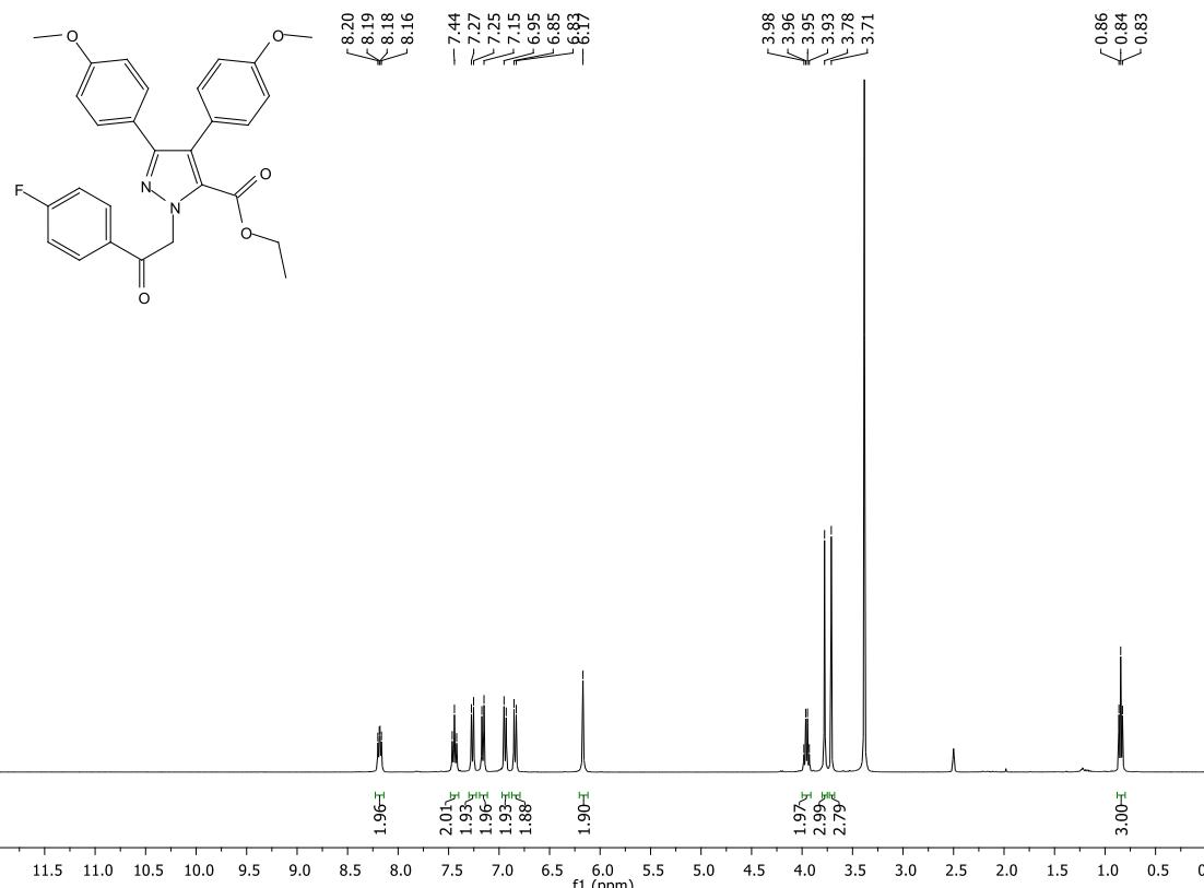
**Figure S82.**  $^1\text{H}$  NMR spectrum (400 MHz, DMSO- $d_6$ ) of ethyl 1-[2-(4-fluorophenyl)-2-oxoethyl]-3,4-bis(4-methoxyphenyl)-1*H*-pyrazole-5-carboxylate (**6h**).
