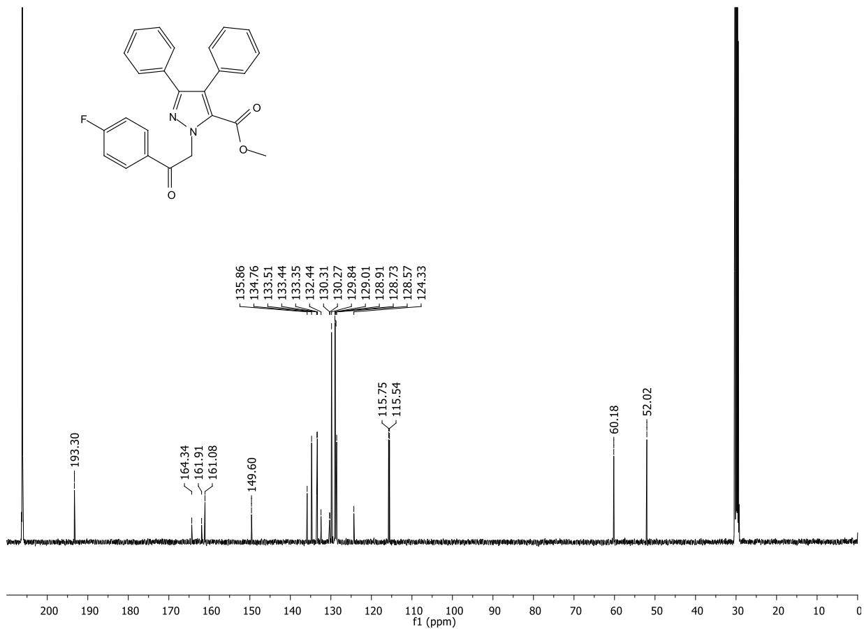
**Figure S130.** <sup>13</sup>C NMR spectrum (101 MHz, acetone-*d*<sub>6</sub>) of methyl 1-[2-(4-fluorophenyl)-2-oxoethyl]-3,4-diphenyl-1*H*-pyrazole-5-carboxylate (**7c**).
