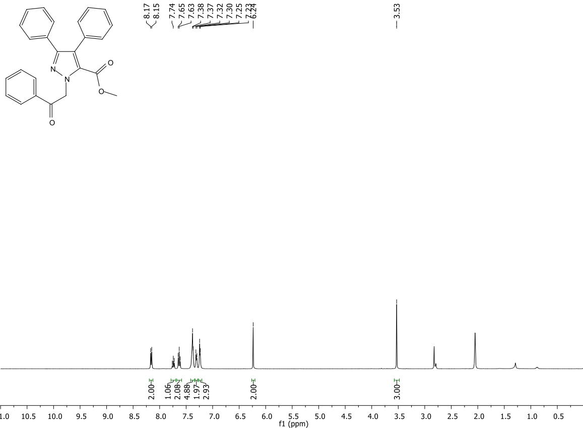
**Figure S121.** <sup>1</sup>H NMR spectrum (400 MHz, acetone-*d*<sub>6</sub>) of methyl 1-(2-oxo-2-phenylethyl)-3,4-diphenyl-1*H*-pyrazole-5-carboxylate (**7a**).
