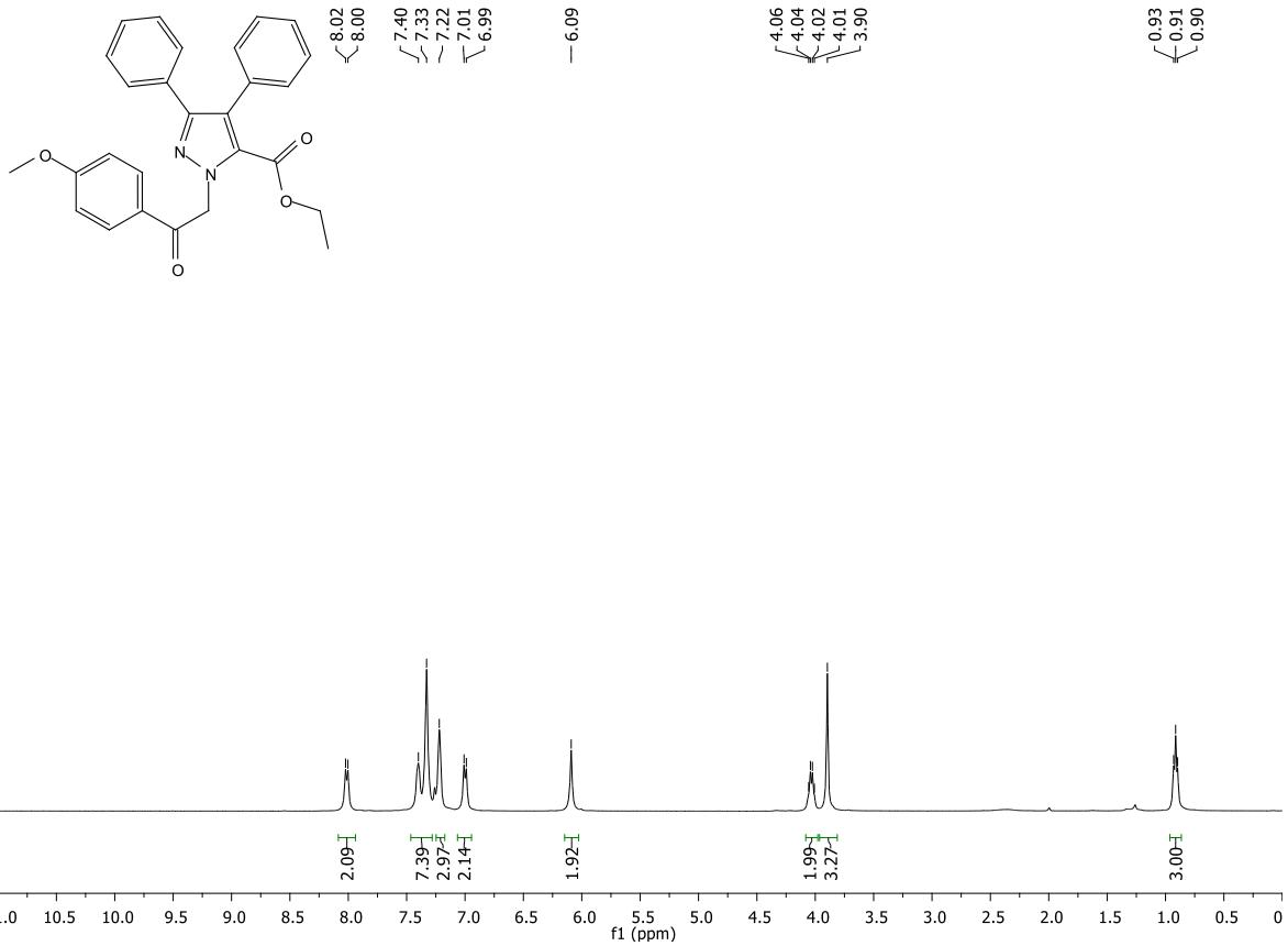
**Figure S57.**  $^1\text{H}$  NMR spectrum (400 MHz,  $\text{CDCl}_3$ ) of ethyl 1-[2-(4-methoxyphenyl)-2-oxoethyl]-3,4-diphenyl-1*H*-pyrazole-5-carboxylate (**6b**).
