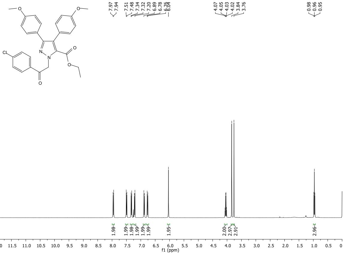
**Figure S87.** <sup>1</sup>H NMR spectrum (400 MHz, CDCl<sub>3</sub>) of ethyl 1-[2-(4-chlorophenyl)-2-oxoethyl]-3,4-bis(4-methoxyphenyl)-1*H*-pyrazole-5-carboxylate (6i).
