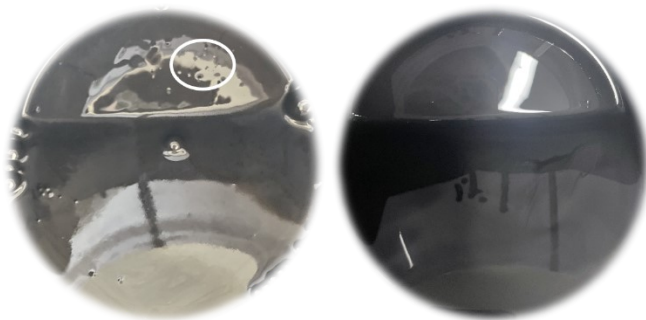
Fig S3. Ball milling causes the disappearance of large particles in the ink. (left) Before ball milling; (right) After ball milling.
