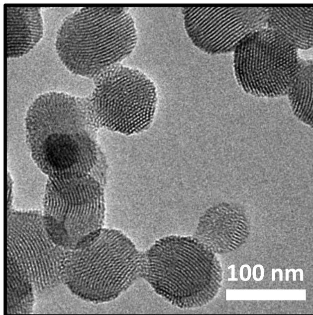
**Figure S2.** TEM image of MSN-PEG after ultrasound treatment and heating at 50 °C for 30 min.
