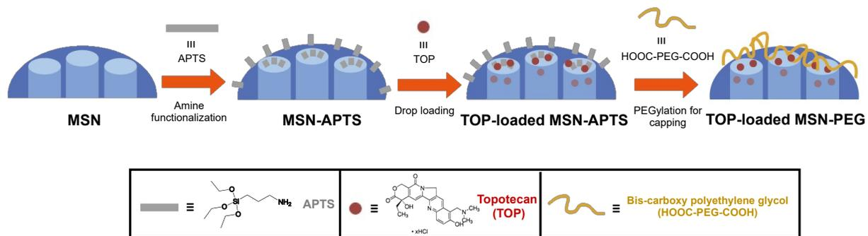
**Scheme S1:** Synthesis of ultrasound-responsive PEGylated mesoporous silica nanoparticles (MSN-PEG)
