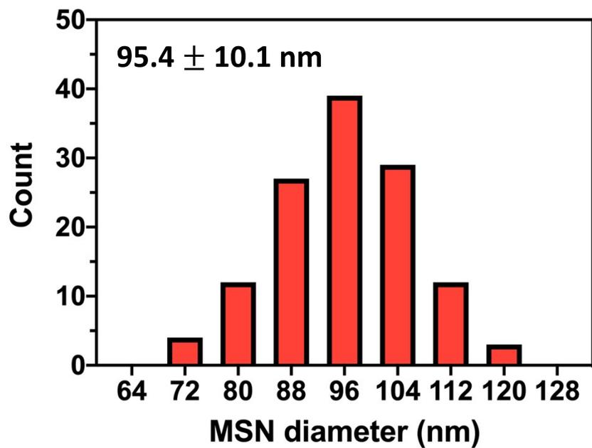
**Figure S1.** Size distribution of  $95.4 \pm 10.1$  nm mesoporous silica nanoparticle (MSN) calculated from TEM images.
