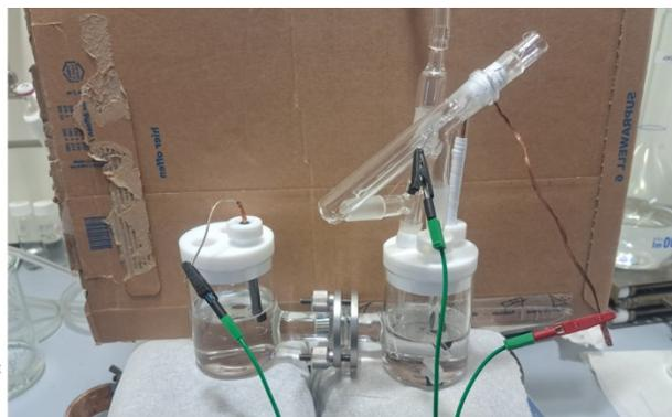
**Figure S16.** Schematic representation of the H-cell (left) and picture of the H-cell (right).
