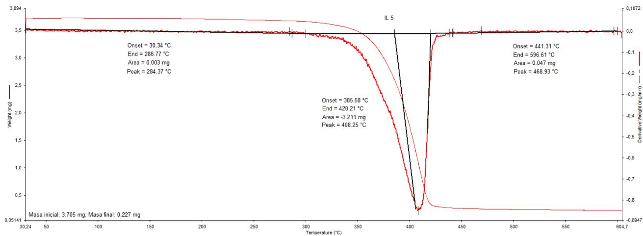
Figure S6: M8 - TGA thermogram.
