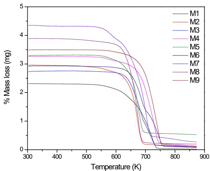
Figure S3: TGA thermograms for the reciprocal binary mixtures of ILs.
