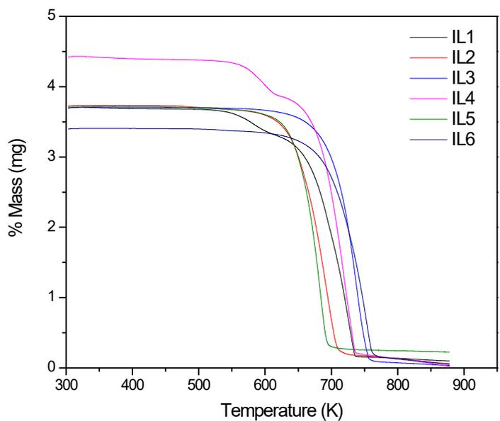
Figure S2: TGA thermograms for the binary mixtures of ILs.
