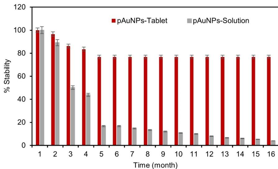
**Figure S 8.** The stability analyses of pAuNPs-Tablet show ultra-stable properties compared to pAuNPs-Solution over a period of ~16 months.
