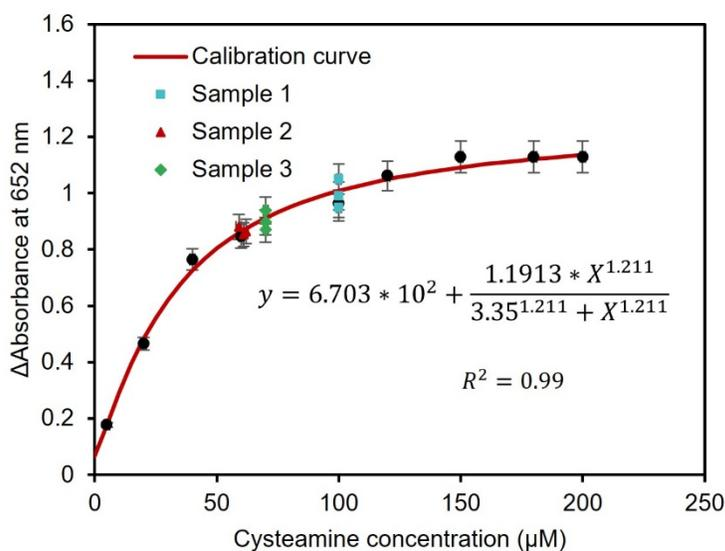
**Figure S 7.** Analytical performance of the tablet-based sensor in real human serum samples. The calibration curve was attained by testing the sensor with the known concentrations of 60, 70, and 100  $\mu\text{M}$  cysteamine in real human serum samples. A Hill function was fit to the whole data with an  $R^2 > 0.99$ , showing the compatibility of the data with a standard saturation model. Each data point is the mean  $\pm$  standard deviation of the replications ( $n = 3$ )
