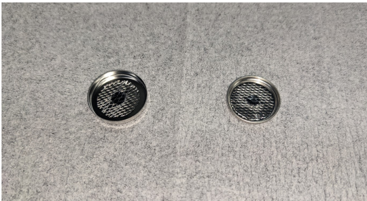
Fig. S4 Photo image of electrode pellets crimped to mesh current collector and coin-type cell parts.
