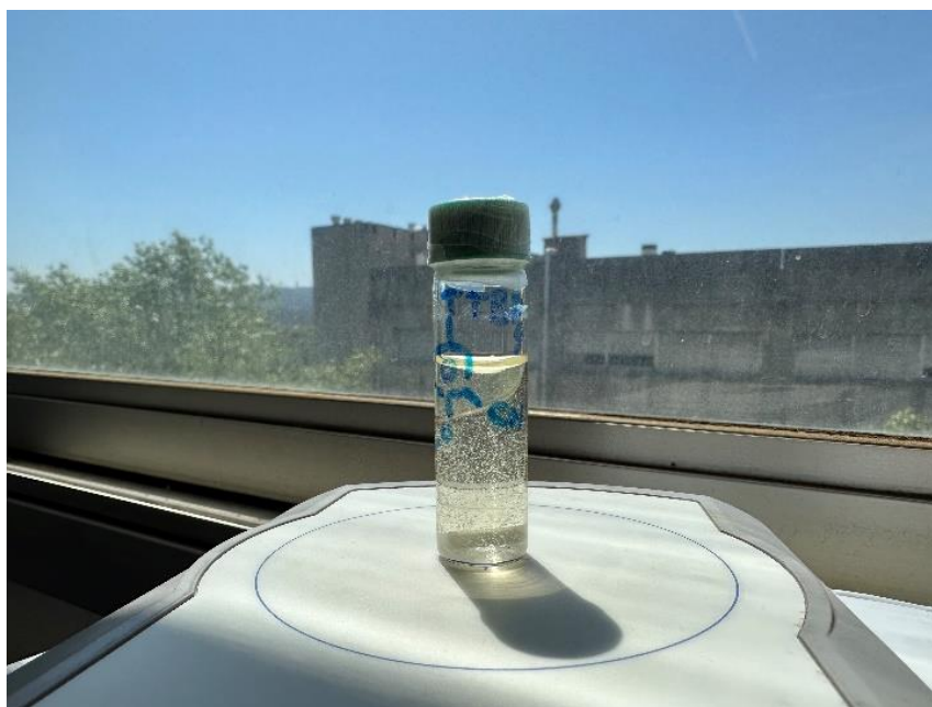
Figure S2. Setup for the sun-light driven synthesis of 4 .
