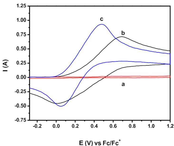
Cyclic voltammograms in 0.1 M  $\text{LiClO}_4$  in MeCN solution of (a) 1-phenylethanol (2.0 mmol), (b) ACT (**1**, 0.4 mmol) and (c) 1-phenylethanol (2.0 mmol) + ACT (**1**, 0.4 mmol), at a scan rate of  $200 \text{ mV s}^{-1}$ . Working electrode: glassy carbon. Pseudo reference electrode:  $\text{Ag}/\text{Ag}^+$  (ferrocene as internal reference). Counter electrode: Pt plated electrode.
