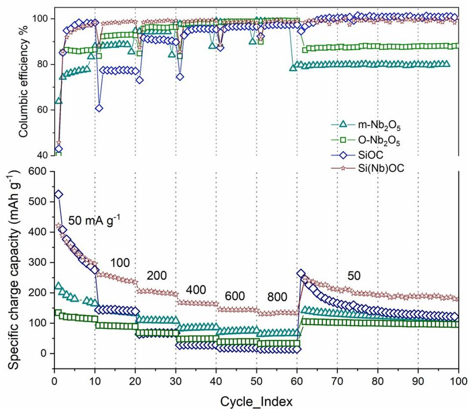
**Fig. S6** Cyclic stability of pure Nb<sub>2</sub>O<sub>5</sub> and as-pyrolyzed Si(Nb)OC composite anodes when cycled asymmetrically at increasing current densities and their respective columbic efficiency
