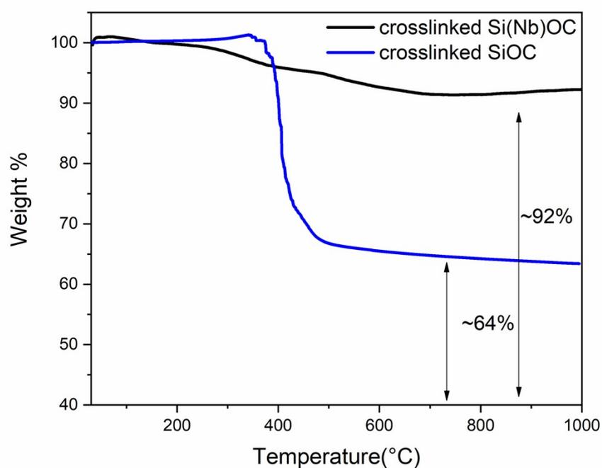
**Fig. S1** Thermogravimetric analysis of crosslinked Si(Nb)OC shows Nb modification improves the stability of Si(Nb)OC composites due to suppressed decomposition of Si-O-C bonds
