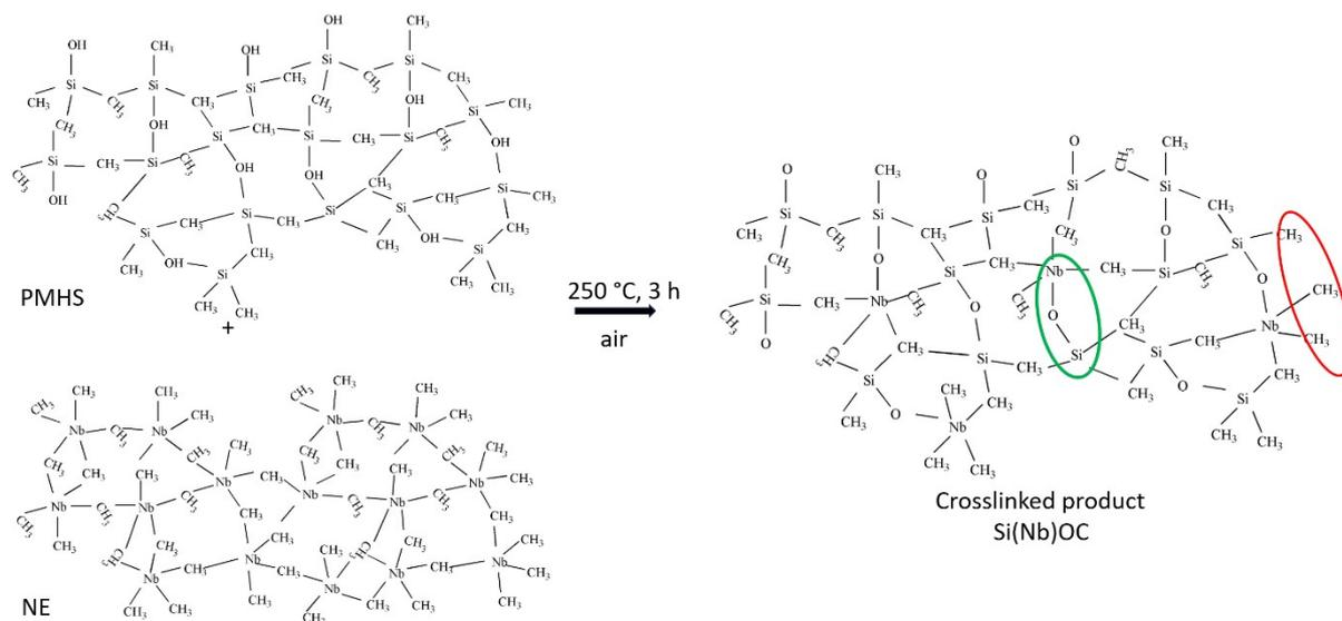
**Fig. S2** Chemical structure of initial precursors and crosslinked product of modified PMHS:NE showing Si-O-Nb linkage (green) and methyl groups (red), subsequent heating which leads to produced in situ segregated carbon and amorphous Si(Nb)OC structure.
