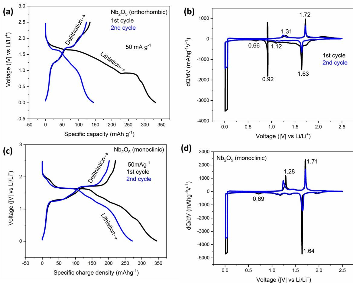
**Fig. S5** Charge-discharge curves and respective differentiated capacity curves of pure Nb<sub>2</sub>O<sub>5</sub> (a-b) orthorhombic Nb<sub>2</sub>O<sub>5</sub> (900 °C) and (c-d) monoclinic Nb<sub>2</sub>O<sub>5</sub> (1200 °C)
