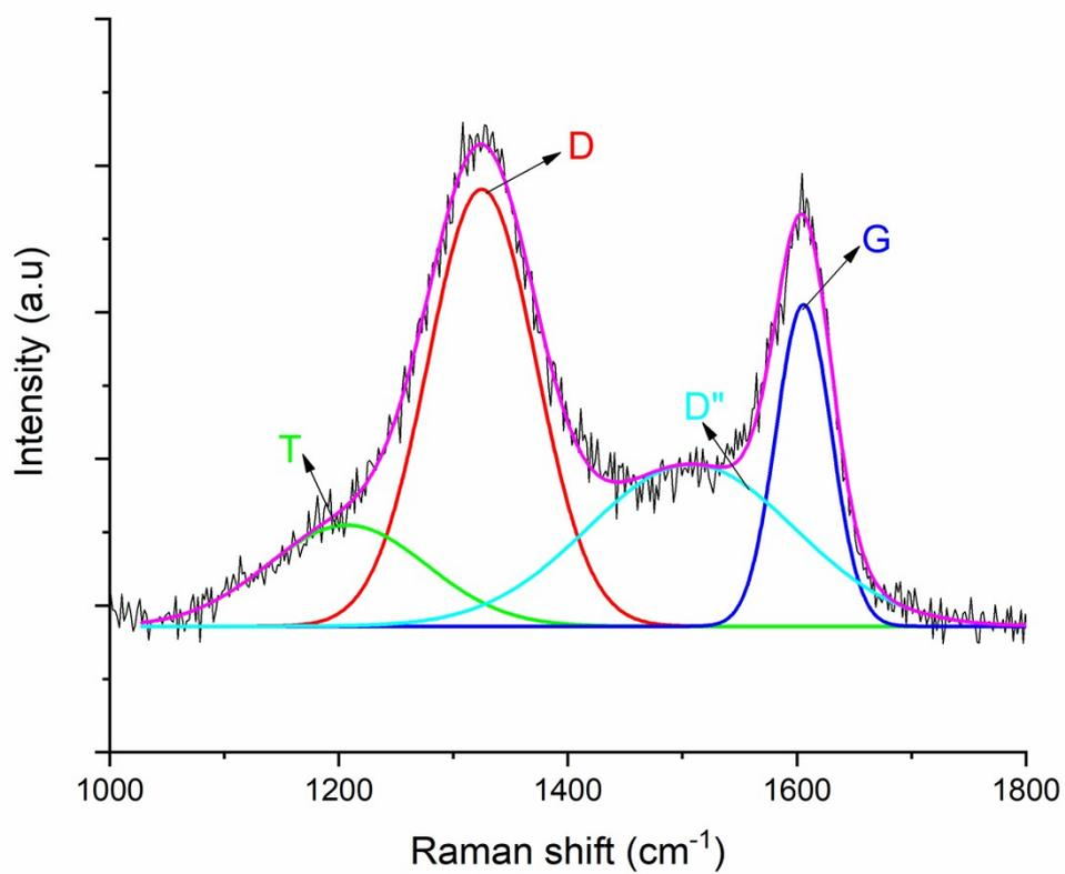
**Fig S4.** Raman spectrum deconvoluted peaks D and G peaks of annealed Si(Nb)OC.
