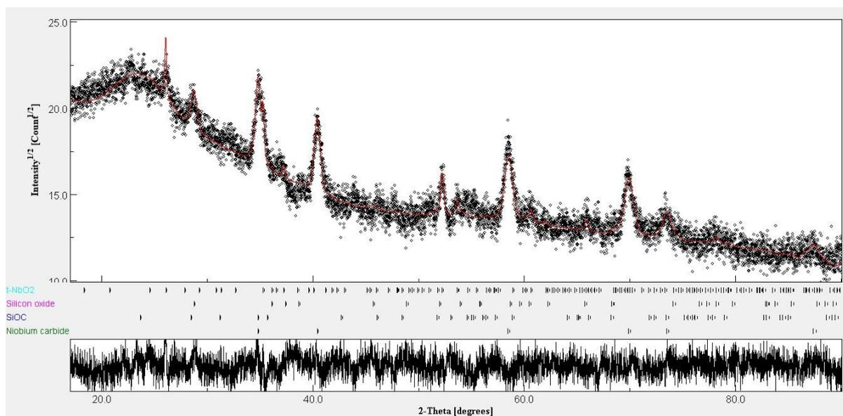
**Fig. S3.** Rietveld refinement of Si(Nb)OC composites using MAUD software
