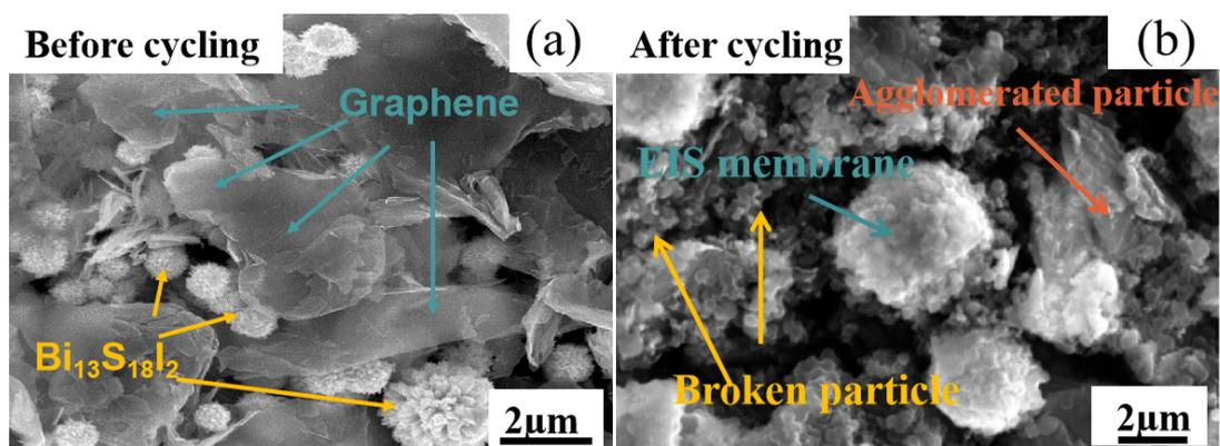
Fig. S2 (a) FE-TEM image of the 150 G/BSI electrode before cycling; (b) FE-TEM images of the 150 G/BSI electrode after 500 cycles.
