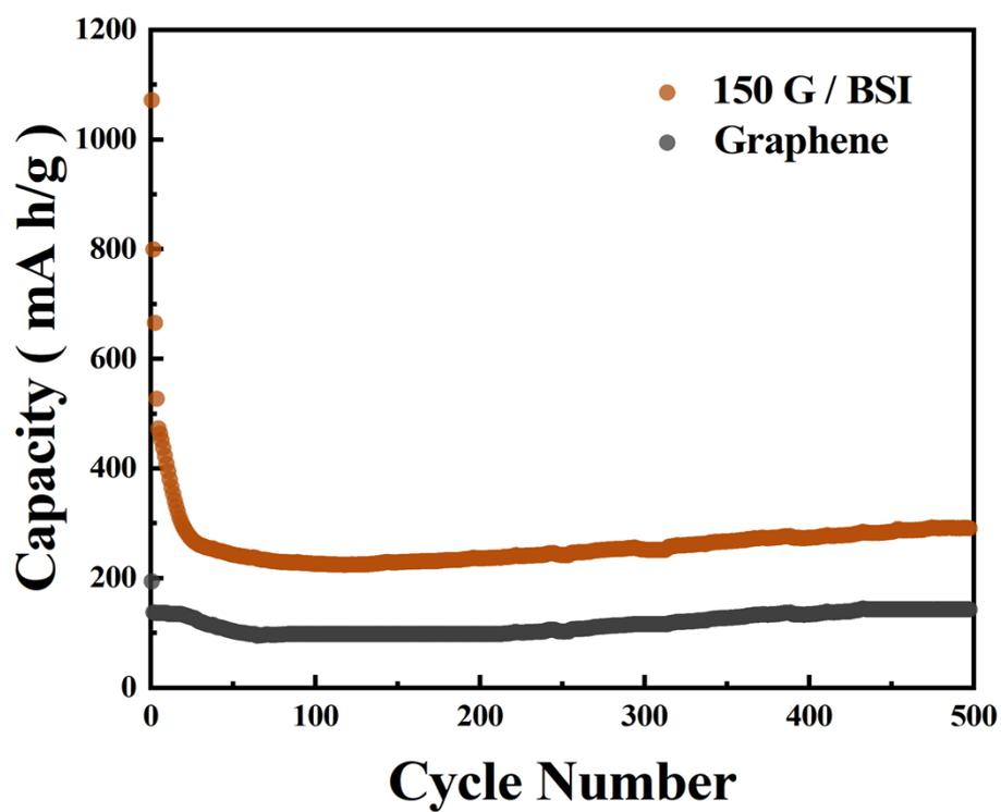
Fig. S4 Long Cycle Performance of Graphene and 150 G / BSI at 0.5 A/g
