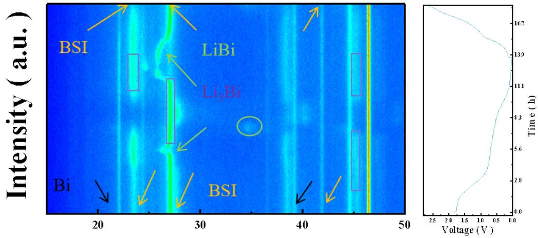
Fig. S7 In situ XRD patterns of the 150 G/BSI electrode during the first cycle and the corresponding discharge and charge curves.
