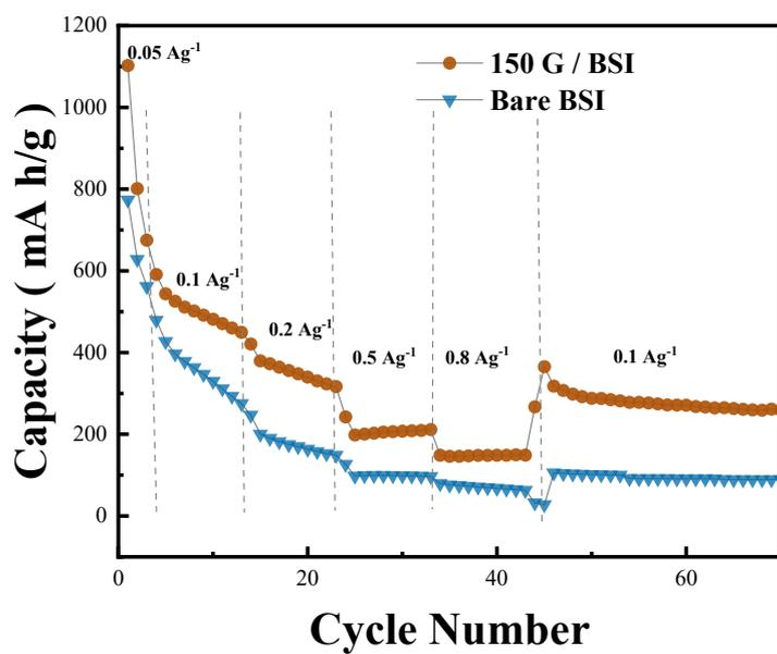
Fig. S5 Rate performance at different current densities of Bare BSI and 150 G/BSI.
