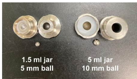
Figure S2. Stainless jar (1.5 mL and 5 ml) and ball (5 mm and 10 mm) used in this study.
