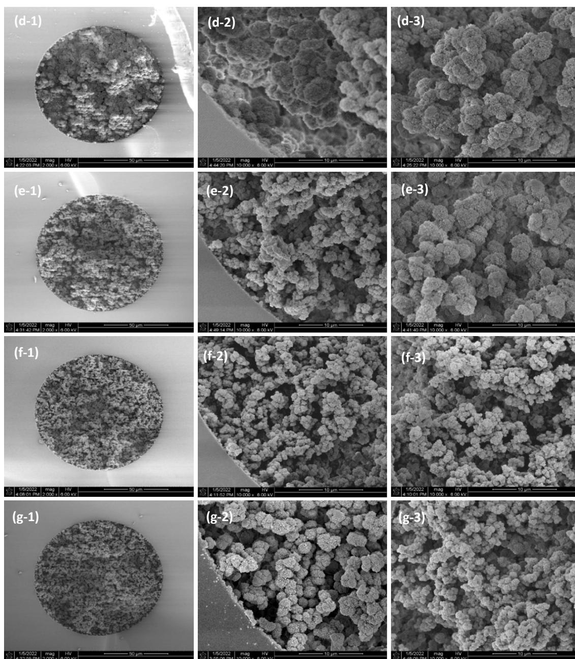
**Fig. S3** Morphologies of various monoliths prepared with the recipes d-g. Numbers 1, 2 and 3 represent the morphology of monolith observed at different locations, 1 refers to the cross section, 2 refers to the tube wall, and 3 refers to the center of capillary monolithic column.
