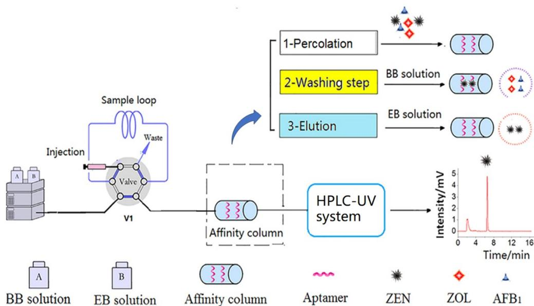
**Fig. S1** Process of online recognition of DA using affinity monolith coupled with HPLC-UV
