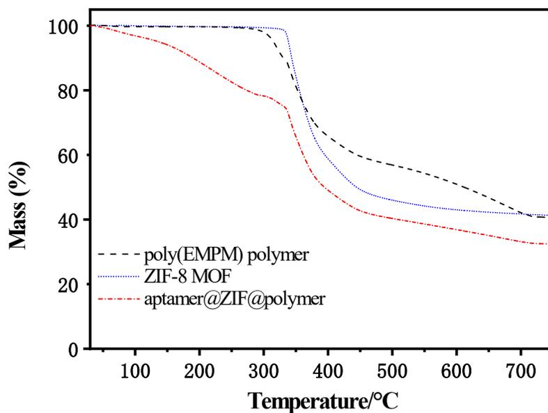
**Fig. S5** TGA of ZIF-8, poly (EMPM) polymer and polyEMPM@ZIF-8@aptamer monolith
