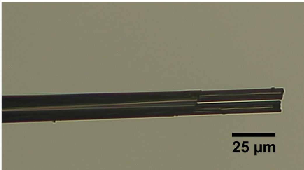
Figure S1: Optical microscope image of double-bore CFM.
