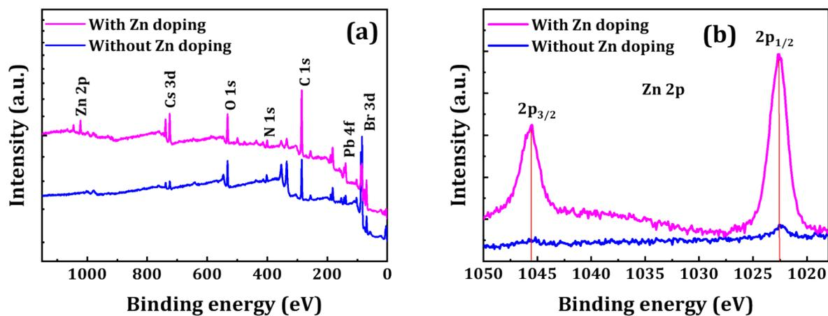
Figure S2: (a) Core XPS pattern of CsPbBr<sub>3</sub> NCs without Zn and with Zn-doping, and (b) high-resolution XPS patterns of Zn 2p chemical state, as shown in legends.
