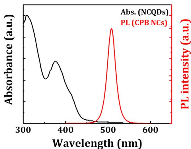
Figure S7: Absorption and PL spectra of the acceptor (NCQDs) and donor (CsPbBr<sub>3</sub> NCs) respectively as shown in legends.
