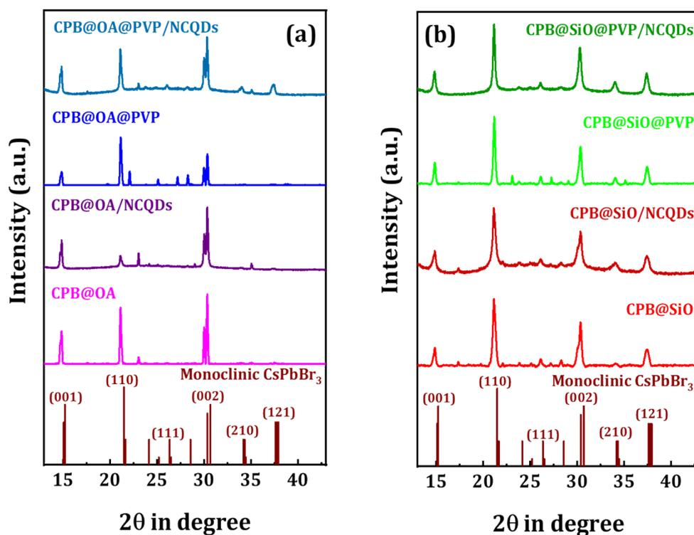
Figure S6: XRD Diffraction patterns of (a) CPB@OA and CPB@OA@PVP, (b) CPB@SiO and CPB@SiO@PVP NCs with and without NCQDs as marked in the Figure.
