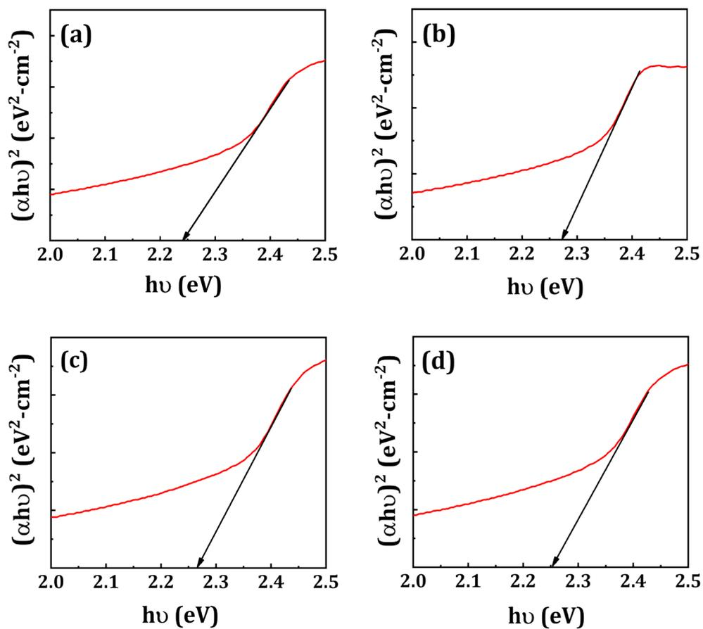
**Figure S1:** Tauc plots of (a) CPB@OA, (b) CPB@OA@PVP, (c) CPB@SiO, and (d) CPB@SiO@PVP NCs.
