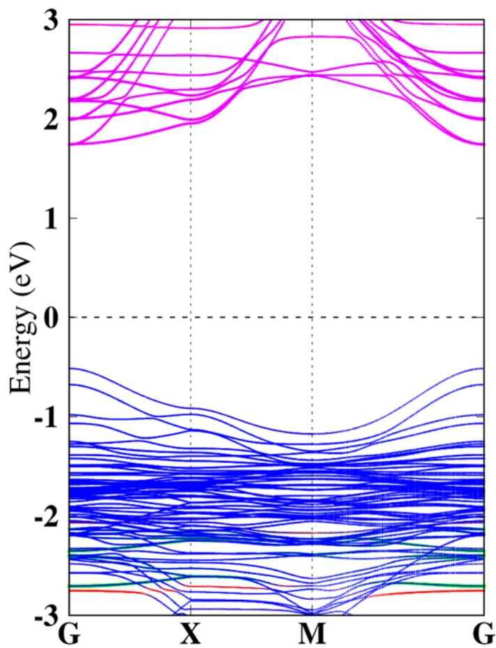
**Figure S8:** Projected band structures of CsPbBr<sub>3</sub> slab with NH<sub>3</sub> molecule.
