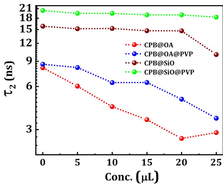
**Figure S5:** Decay component ( $\tau_2$ ) of NCs over addition of different volumes of NCQDs as shown in legend.
