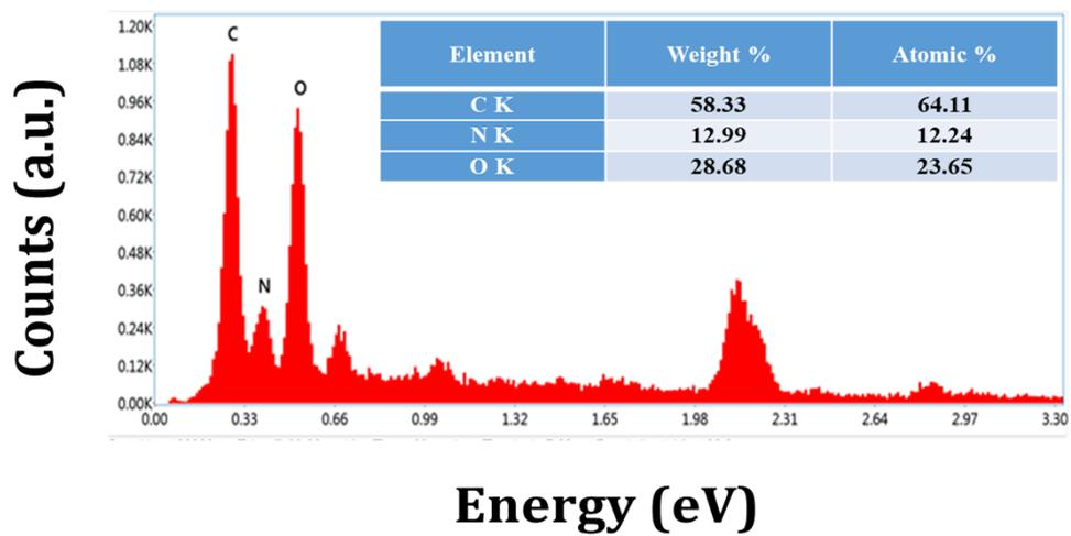
**Figure S4:** EDS spectrum of NCQDs film showing all the elements present on the surface. Inset: EDS data obtained from FESEM image showing both the weight and atomic percentage of different elements.
