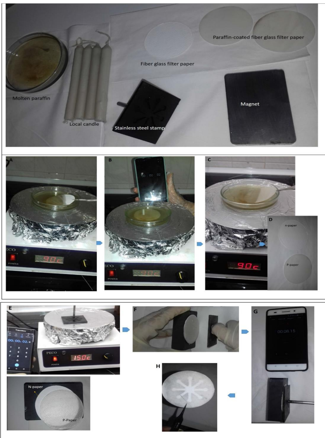
Scheme S1. Materials and equipment (I), and the process (II) of \mu PAD fabrication. Wax melting at 90 degrees Celsius, followed by filter paper, put it flat. (A), and left it for 2 s (B), afterwards, the filter paper was taken out (C) to prepare a paraffinic paper (D). The locally machined steel stamp was heated at 150 °C for 25° and the p-paper was put on the n-paper (E), before stamping (F). The stamping step was performed during 8 s (G) to prepare the proposed \mu PAD.
