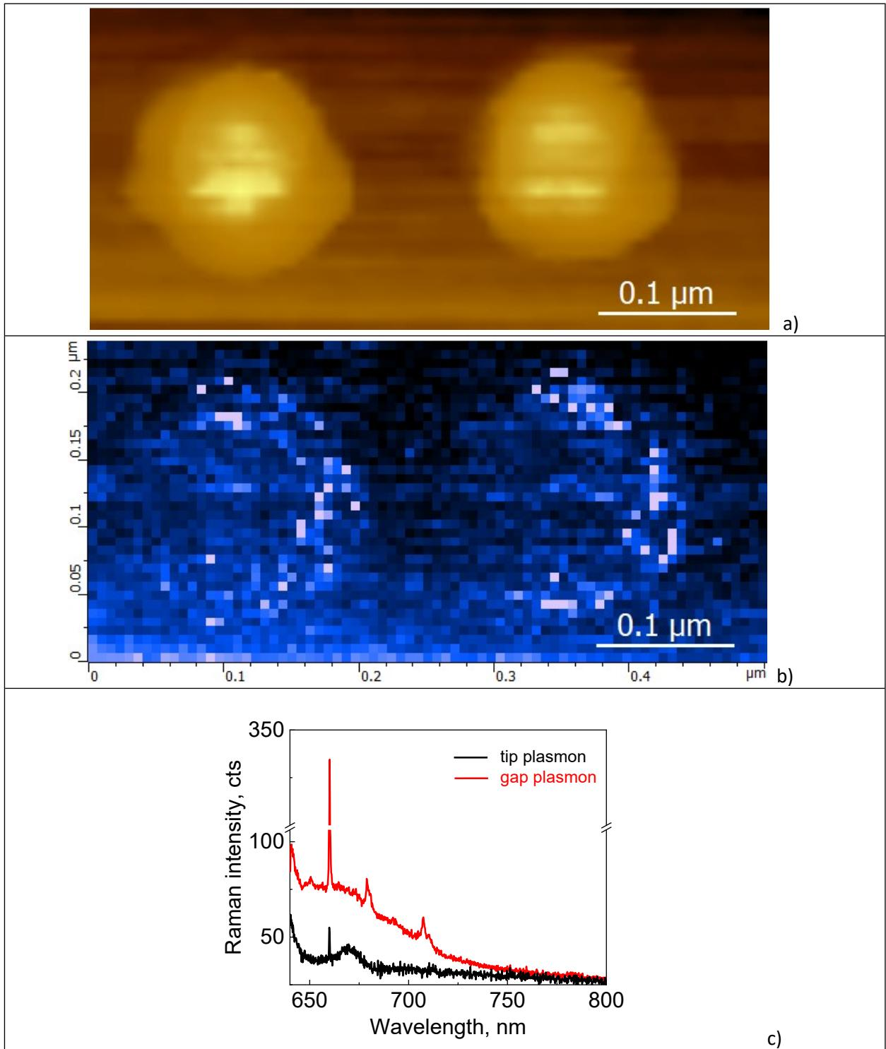
**Fig.S3** (a)- AFM and (b) TERS- images of bare nanodisks measured by Ag tip. (c) Raman spectrum of Ag tip apex and TERS spectrum Au nanoclusters measured in gm-TERS conditions
