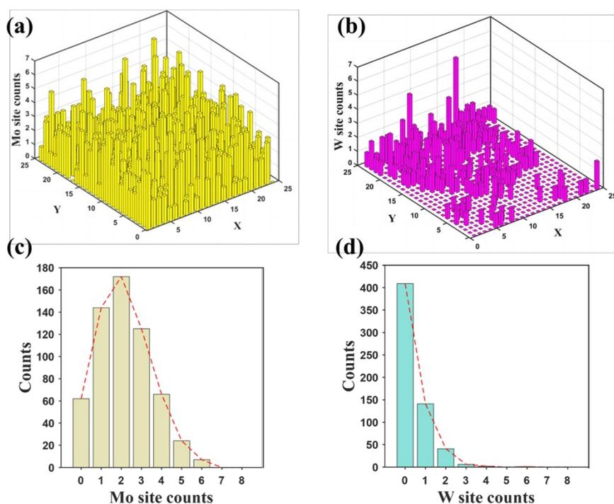
Figure S6. STEM analysis of monolayer  $\text{Mo}_x\text{W}_{(1-x)}\text{S}_{2y}\text{Se}_{2(1-y)}$  alloy. (a-b) The site distribution histograms of Mo and W in monolayer  $\text{Mo}_{0.82}\text{W}_{0.18}\text{S}_{0.28}\text{Se}_{1.72}$  alloy, respectively. The image was divided into  $25 \times 25$  parts. (c-d) The corresponding statistical histograms of Mo-site and W-site counts in each part of STEM image.
