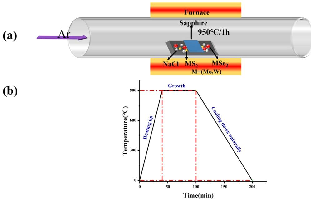
Figure S1. (a) Schematic illustration of the single-heating-zone furnace for the synthesis of monolayer  $\text{Mo}_x\text{W}_{(1-x)}\text{S}_{2y}\text{Se}_{2(1-y)}$  alloys. (b) Temperature profiles of the samples during growth.
