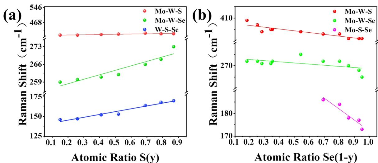
Figure S3. (a) Composition-dependent Raman frequencies of  $\text{Mo}_x\text{W}_{(1-x)}\text{S}_{2y}\text{Se}_{2(1-y)}$  with different weight ratios of  $\text{MoS}_2$  and  $\text{WSe}_2$  as growth sources. (b) Composition-dependent Raman frequencies of  $\text{Mo}_x\text{W}_{(1-x)}\text{S}_{2y}\text{Se}_{2(1-y)}$  with different weight ratios of  $\text{MoSe}_2$  and  $\text{WS}_2$  as growth sources.
