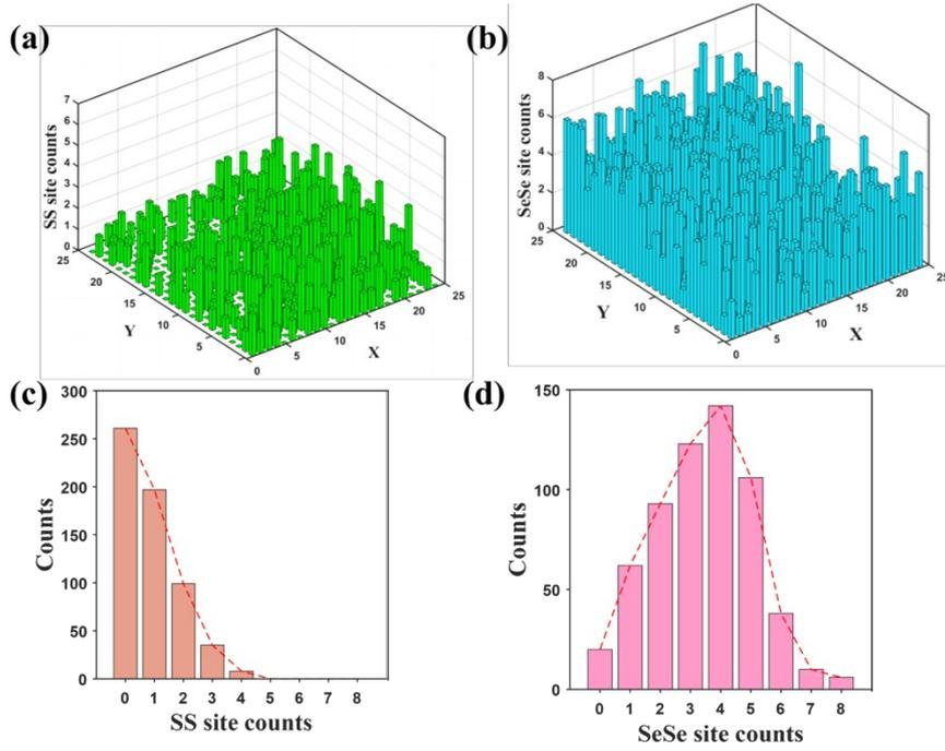
Figure S7. STEM analysis of monolayer  $\text{Mo}_x\text{W}_{(1-x)}\text{S}_{2y}\text{Se}_{2(1-y)}$  alloy. (a-b) The site distribution histograms of SS and SeSe in monolayer  $\text{Mo}_{0.82}\text{W}_{0.18}\text{S}_{0.28}\text{Se}_{1.72}$  alloy, respectively. The image was divided into  $25 \times 25$  parts. (c-d) The corresponding statistical histograms of SS-site and SeSe-site counts in each part of STEM image.
