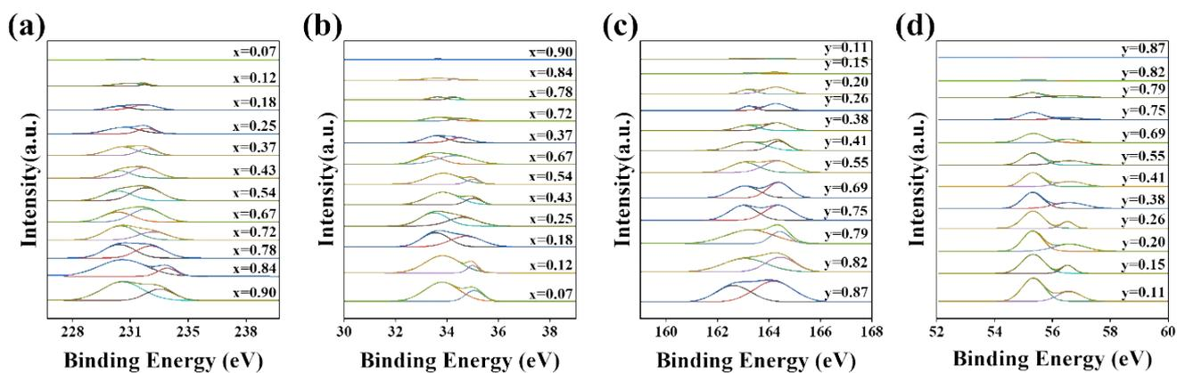
Figure S5. Composition-dependent XPS spectra of monolayer  $\text{Mo}_x\text{W}_{(1-x)}\text{S}_{2y}\text{Se}_{2(1-y)}$  alloys with different weight ratios of  $\text{MoSe}_2$  and  $\text{WS}_2$  as growth source. (a) Mo 3d, (b) W 4f, (c) S 2p and (d) Se 3d.
