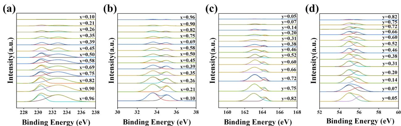
Figure S4. Composition-dependent XPS spectra of monolayer  $\text{Mo}_x\text{W}_{(1-x)}\text{S}_{2y}\text{Se}_{2(1-y)}$  alloys with different weight ratios of  $\text{MoS}_2$  and  $\text{WSe}_2$  as growth source. (a) Mo 3d, (b) W 4f, (c) S 2p and (d) Se 3d.
