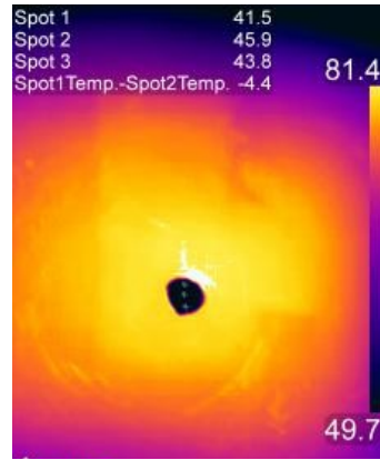
Fig. S6 SA aerogel (2%) thermal image (heating after 90S)
