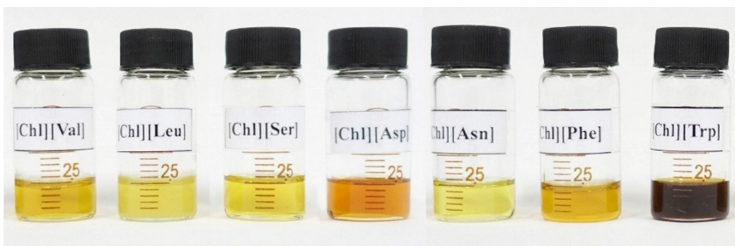
Fig. S2. The seven choline amino acid ionic liquids ([Chl][AA] ILs) synthesized in this study.
