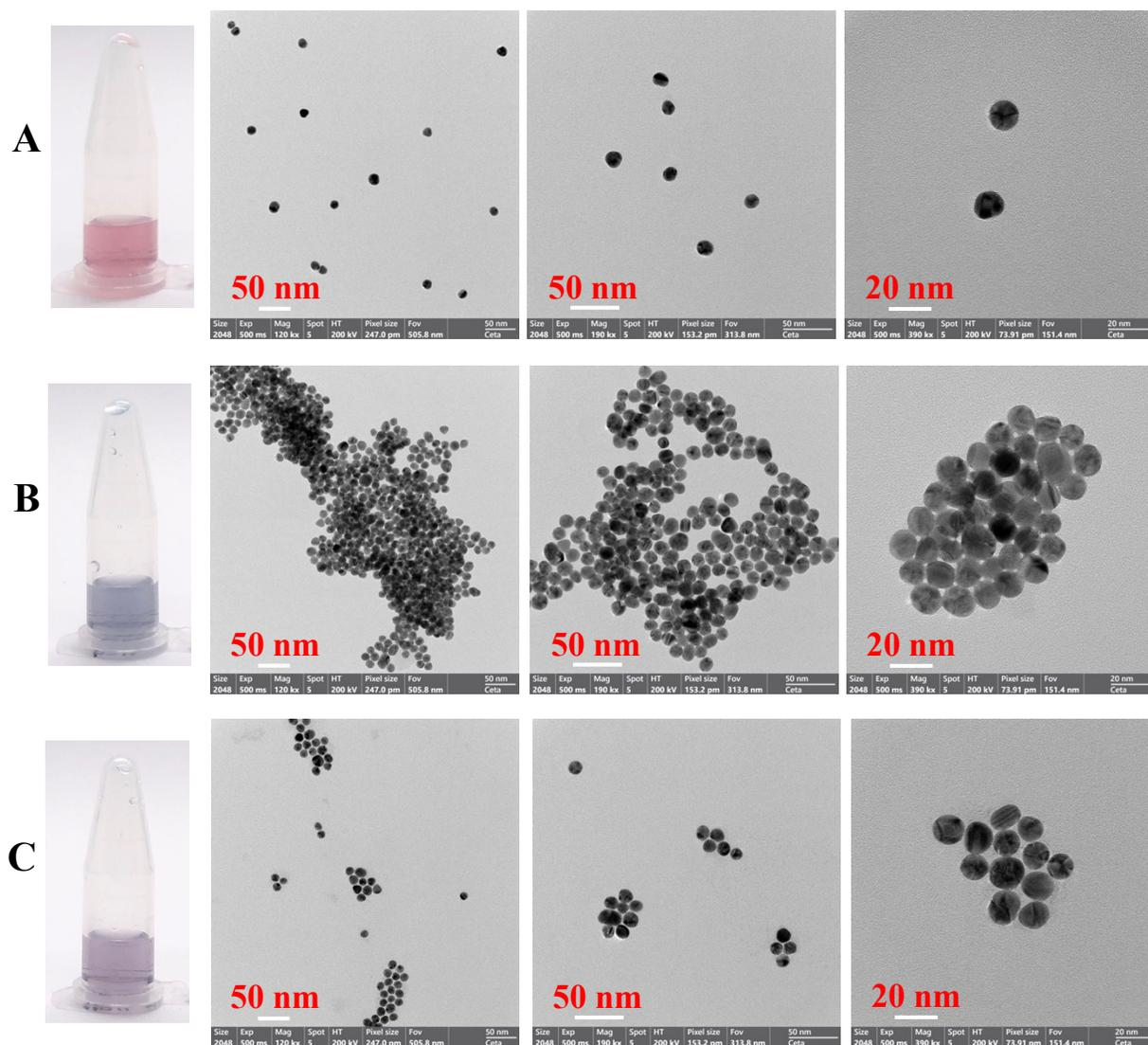
**Fig. S1** Color and FE-TEM images of (A) AuNPs@Cyst without Hcy (blank solution), (B) AuNPs@Cyst with Hcy (aggregation) and (C) AuNPs@Cyst with Hcy after heating at 90 °C for 10 min (de-aggregation). Magnitudes of FE-TEM were 120 kx, 190 kx and 390 kx, respectively.
