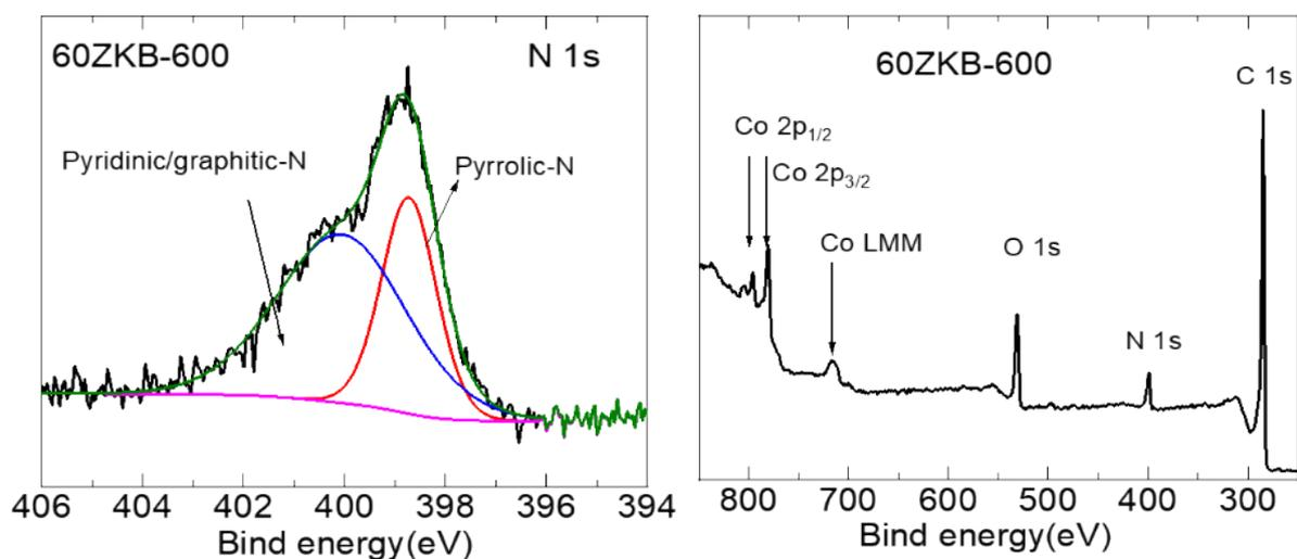
Figure S6. High-resolution XPS N 1s spectra with deconvoluted peak fittings (left) and overall survey spectra (right) for 60ZKB-600 sample. The conversion of ligand pyrrolic-N component to pyridinic-N (at  $\sim 398.7$  eV) and combined pyrrolic/graphitic-N ( $\sim 400$  eV) can be seen (see main ref. 8,15,22,23). The overall survey spectra account for about 82.7 at% C, 9.27 at% O, 5.72 at% N and 2.46 at% Co in the sample.
