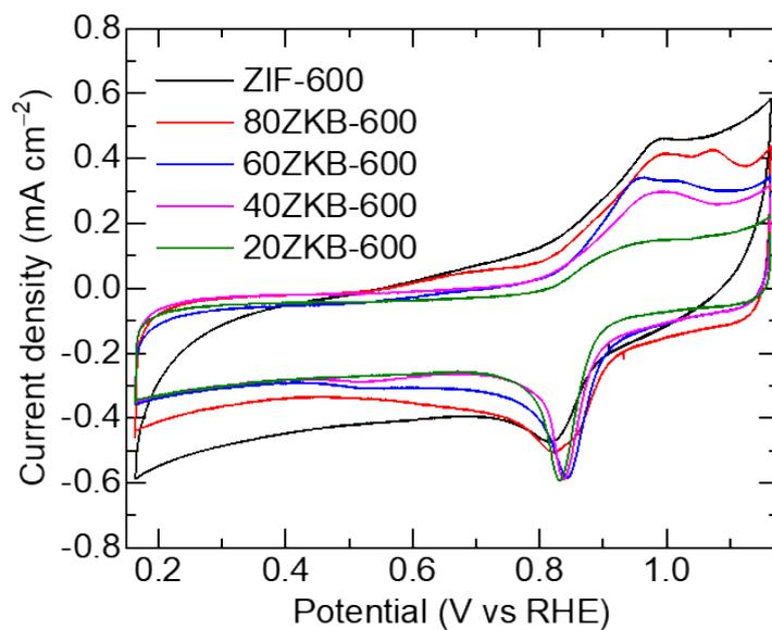
Figure S1. CV curves of xZKB-600 and ZIF-600 samples, measured in 0.1 M KOH at 10 mV s<sup>-1</sup> scan rate.
