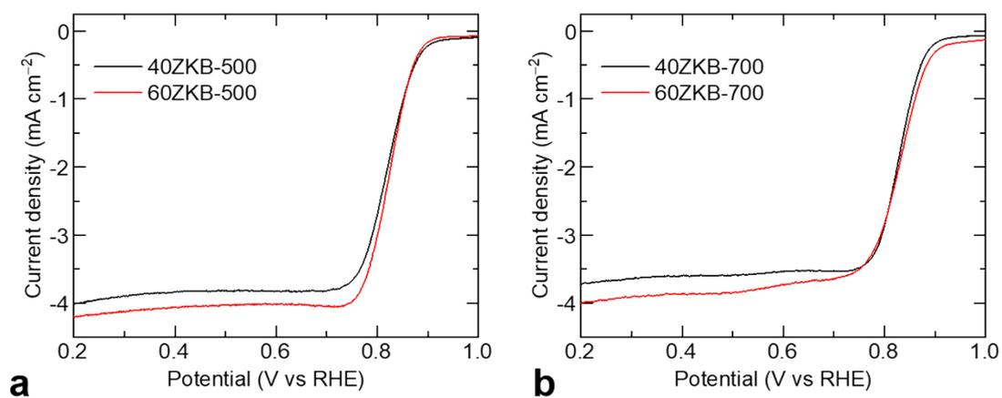
Figure S2. Comparative LSV curves of 40ZKB and 60ZKB samples thermolyzed at a) 500 °C and b) 700 °C. This shows better ORR performance of thermolyzed 60ZKB samples over thermolyzed 40ZKB samples.
