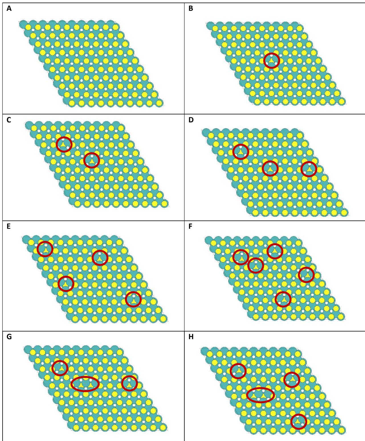
*Supporting Figure 3: Top-down view of  $\text{MoS}_2$  surfaces with defects. Each structure contains three layers of  $\text{MoS}_2$  and 20 Å of vacuum space above the surface. Defects are only on the top basal surface. A) 0 defects, B) 1 defect, C) 2 defects, D) 3 defects, E) 4 defects (none adjacent), F) 5 defects (none adjacent), G) 4 defects (2 adjacent), H) 5 defects (2 adjacent). Colors: yellow S, teal Mo*
