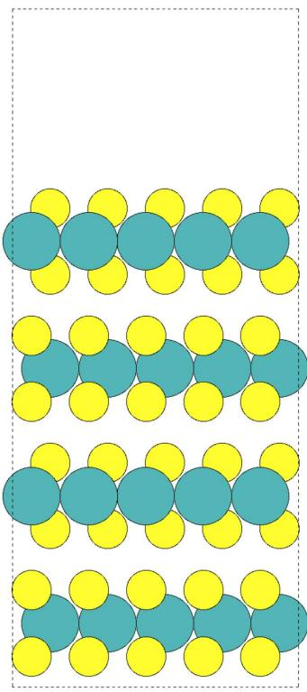
*Supporting Figure 2: Visualization of MoS<sub>2</sub> structure used for layer separation calculations. The system is periodic in all directions. Colors: yellow S, teal Mo*
